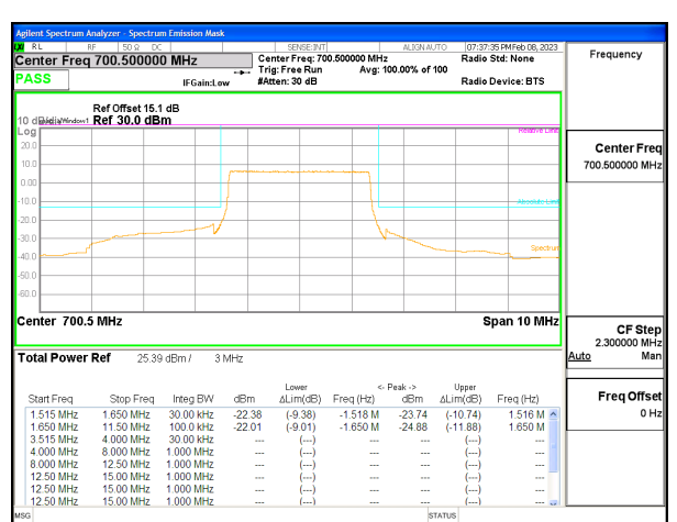
LTE B12 3MHz QPSK Low Channel RB15-0, ID:25780
