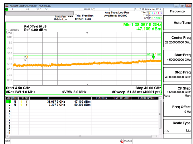
5G NR n48 10MHz BPSK High Channel RB1-23 (4.5G to 40G), ID:12482
