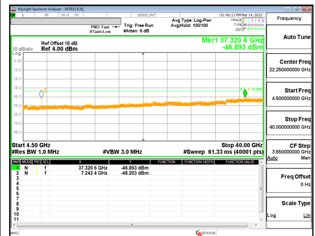
5G NR n48 10MHz BPSK Mid Channel RB1-1 (4.5G to 40G), ID:12482
