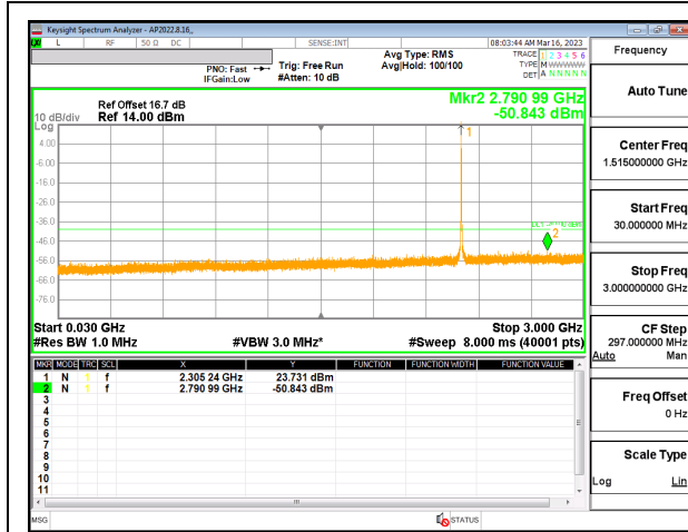
5G NR n30 5MHz QPSK Low Channel RB1-0 (30MHz to 3GHz), ID:32061
