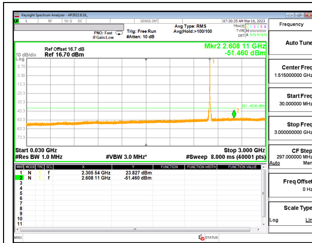
5G NR n30 10MHz QPSK Mid Channel RB1-0 (30MHz to 3GHz), ID:32061
