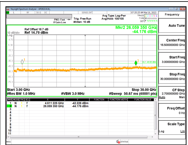
5G NR n30 10MHz QPSK Middle Channel RB1-0 (3G to 26G) ID:32061
