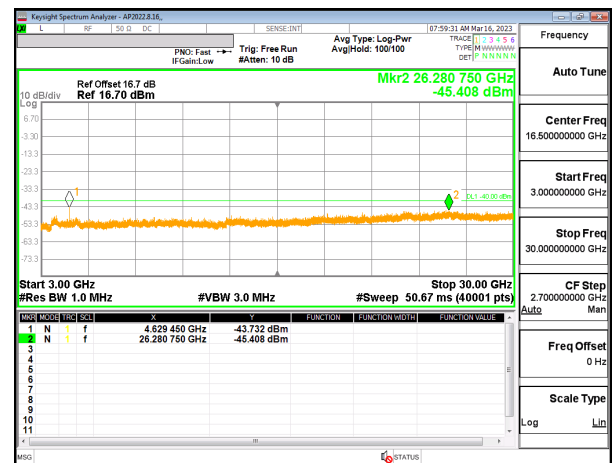
5G NR n30 5MHz QPSK High Channel RB1-0 (3G to 26G) ID:32061
