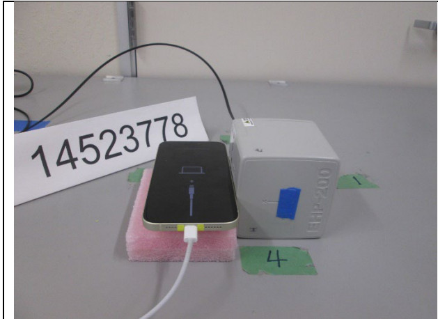
S1, RF Exposure Setup Photo
