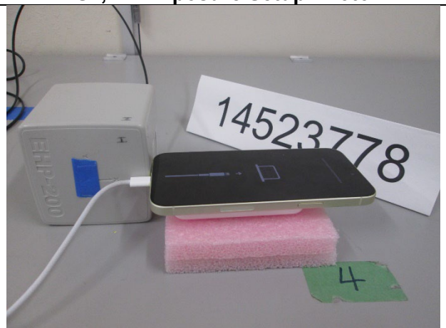
S4, RF Exposure Setup Photo
