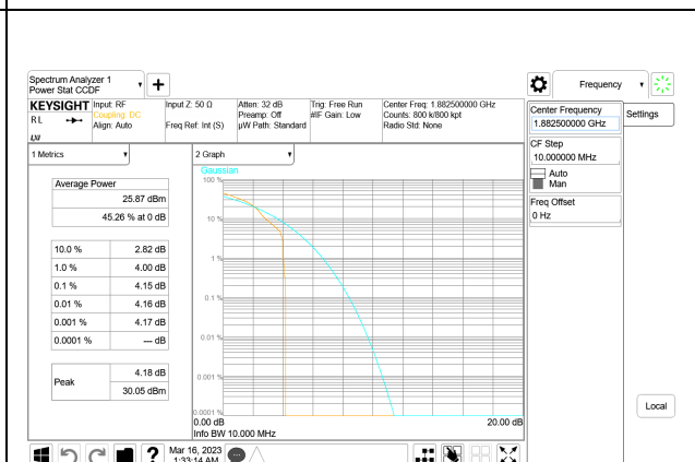
LTE B2 5MHz 16QAM Middle Channel, ID:28567
