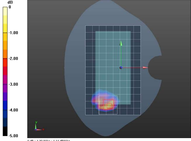
Frequency: 831.5 MHz; Duty Cycle: 1:1; Room Ambient Temperature: 24.0°C; Liquid Temperature: 23.0°C Medium parameters used (interpolated): f = 831.5 MHz;  $\sigma$  = 0.905 S/m;  $\varepsilon_r$  = 40.631;  $\rho$  = 1000 kg/m<sup>3</sup> Dasy Configuration:
