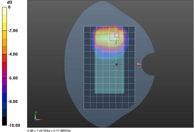
Frequency: 2535 MHz; Duty Cycle: 1:1; Room Ambient Temperature: 24.0°C; Liquid Temperature: 23.0°C Medium parameters used: f = 2535 MHz;  $\sigma$  = 1.894 S/m;  $\epsilon_r$  = 40.105;  $\rho$  = 1000 kg/m³ Dasy Configuration:
