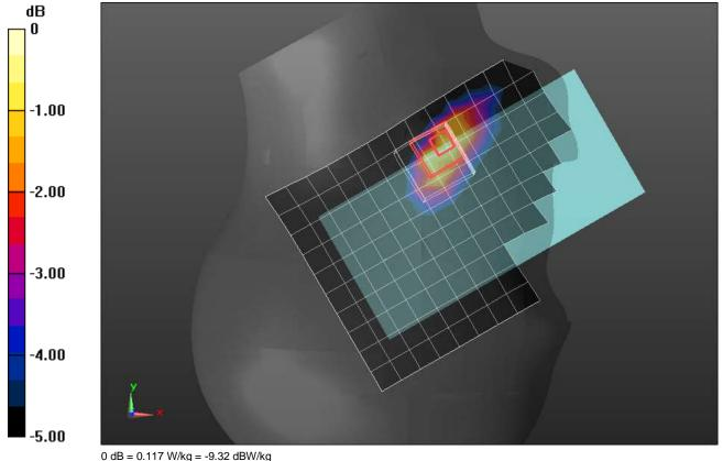
Frequency: 2489.2 MHz; Duty Cycle: 1:1.59956; Room Ambient Temperature: 24.0°C; Liquid Temperature: 23.0°C Medium parameters used: f = 2490 MHz;  $\sigma = 1.808$  S/m;  $\epsilon_r = 37.269$ ;  $\rho = 1000$  kg/m³ Dasy Configuration:
