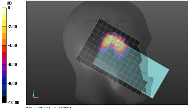
Frequency: 3646.7 MHz; Duty Cycle: 1:1.59956; Room Ambient Temperature: 24.0°C; Liquid Temperature: 23.0°C Medium parameters used (interpolated): f = 3646.7 MHz;  $\sigma = 2.982$  S/m;  $\epsilon_r = 36.162$ ;  $\rho = 1000$  kg/m³ Dasy Configuration:
