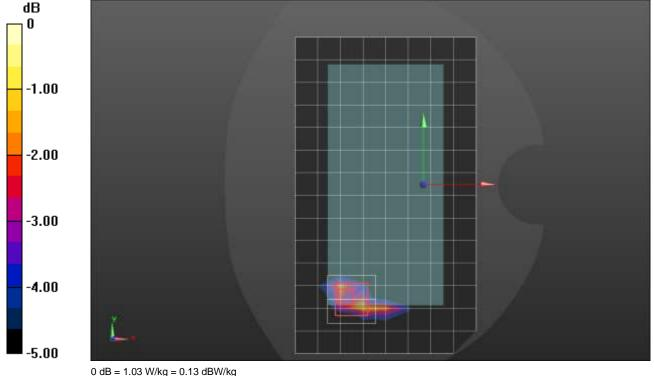
Frequency: 1745 MHz; Duty Cycle: 1:1; Room Ambient Temperature: 24.0°C; Liquid Temperature: 23.0°C Medium parameters used: f = 1745 MHz;  $\sigma = 1.387$  S/m;  $\varepsilon_r = 38.733$ ;  $\rho = 1000$  kg/m<sup>3</sup> Dasy Configuration:
