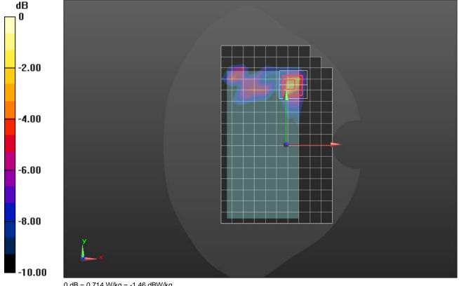
Frequency: 3840 MHz; Duty Cycle: 1:1; Room Ambient Temperature: 24.0°C; Liquid Temperature: 23.0°C Medium parameters used: f = 3840 MHz;  $\sigma$  = 3.143 S/m;  $\epsilon_r$  = 38.909;  $\rho$  = 1000 kg/m³ Dasy Configuration:
