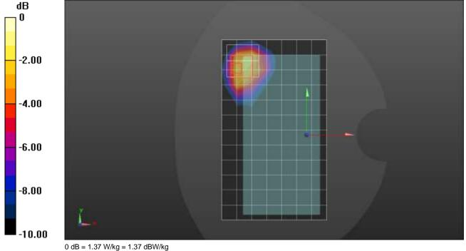
Frequency: 680.5 MHz; Duty Cycle: 1:1; Room Ambient Temperature: 24.0°C; Liquid Temperature: 23.0°C Medium parameters used (interpolated): f = 680.5 MHz;  $\sigma = 0.851$  S/m;  $\epsilon_r = 40.894$ ;  $\rho = 1000$  kg/m³ Dasy Configuration:
