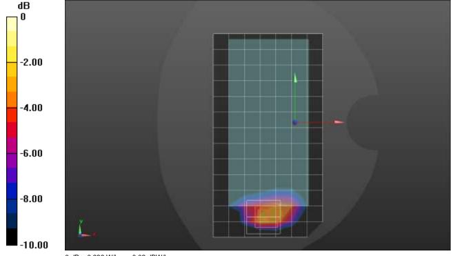
Frequency: 1702.5 MHz; Duty Cycle: 1:1; Room Ambient Temperature: 24.0°C; Liquid Temperature: 23.0°C Medium parameters used (interpolated): f = 1702.5 MHz;  $\sigma = 1.362$  S/m;  $\epsilon_r = 38.809$ ;  $\rho = 1000$  kg/m³ Dasy Configuration:
