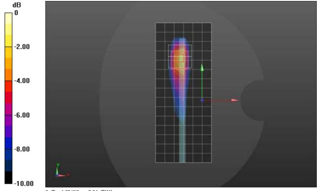
Frequency: 2593 MHz; Duty Cycle: 1:1.59956; Room Ambient Temperature: 24.0°C; Liquid Temperature: 23.0°C Medium parameters used (interpolated): f = 2593 MHz;  $\sigma = 1.913$  S/m;  $\epsilon_r = 37.751$ ;  $\rho = 1000$  kg/m<sup>3</sup> Dasy Configuration:
