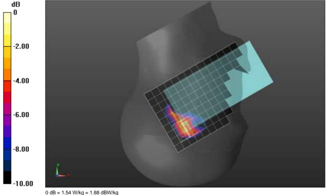
Frequency: 2593 MHz; Duty Cycle: 1:1.59956; Room Ambient Temperature: 24.0°C; Liquid Temperature: 23.0°C Medium parameters used (interpolated): f = 2593 MHz;  $\sigma$  = 1.895 S/m;  $\epsilon_r$  = 37.298;  $\rho$  = 1000 kg/m³ Dasy Configuration:
