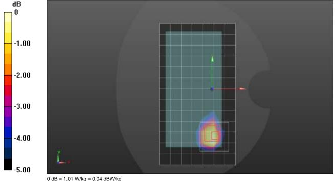
Frequency: 1745 MHz; Duty Cycle: 1:1; Room Ambient Temperature: 24.0°C; Liquid Temperature: 23.0°C Medium parameters used: f = 1745 MHz;  $\sigma$  = 1.385 S/m;  $\epsilon_r$  = 40.583;  $\rho$  = 1000 kg/m³ Dasy Configuration:
