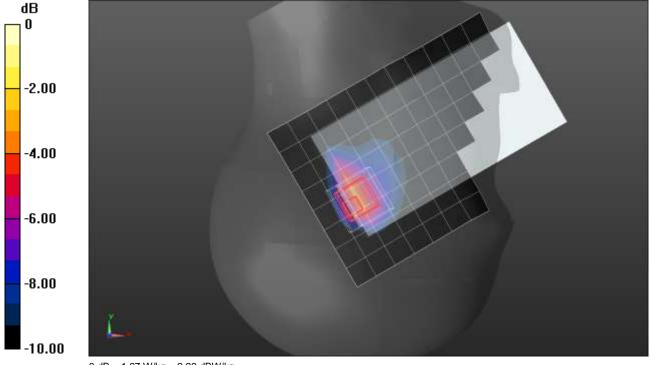
Frequency: 707.5 MHz; Duty Cycle: 1:1; Room Ambient Temperature: 24.0°C; Liquid Temperature: 23.0°C Medium parameters used (interpolated): f = 707.5 MHz;  $\sigma = 0.87 \text{ S/m}$ ;  $\varepsilon_r = 41.411$ ;  $\rho = 1000 \text{ kg/m}^3$ Dasy Configuration:
