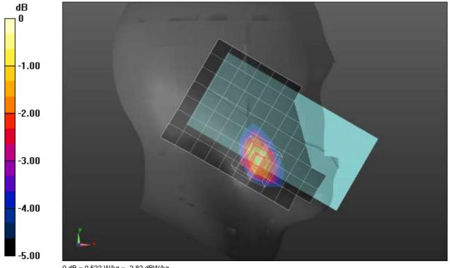
Frequency: 1882.5 MHz; Duty Cycle: 1:1; Room Ambient Temperature: 24.0°C; Liquid Temperature: 23.0°C Medium parameters used (interpolated): f = 1882.5 MHz;  $\sigma = 1.411$  S/m;  $\epsilon_r = 41.604$ ;  $\rho = 1000$  kg/m³ Dasy Configuration:
