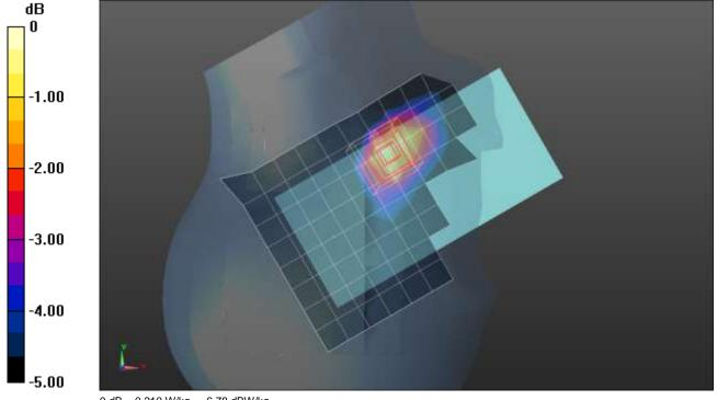
Frequency: 1732.6 MHz; Duty Cycle: 1:1; Room Ambient Temperature: 24.0°C; Liquid Temperature: 23.0°C Medium parameters used (interpolated): f = 1732.6 MHz;  $\sigma$  = 1.399 S/m;  $\epsilon_r$  = 38.926;  $\rho$  = 1000 kg/m³ Dasy Configuration:
