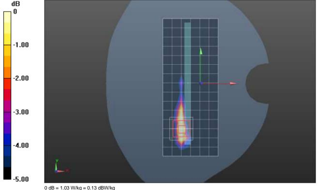
Frequency: 3603.3 MHz; Duty Cycle: 1:1.59956; Room Ambient Temperature: 24.0°C; Liquid Temperature: 23.0°C Medium parameters used (interpolated): f = 3603.3 MHz;  $\sigma = 2.902 \text{ S/m}$ ;  $\epsilon_r = 38.738$ ;  $\rho = 1000 \text{ kg/m}^3$ Dasy Configuration:
