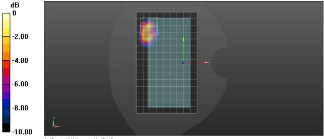
Frequency: 1610.1 MHz; Duty Cycle: 1:2.61096; Room Ambient Temperature: 24.0°C; Liquid Temperature: 23.0°C Medium parameters used (interpolated): f = 1610.1 MHz;  $\sigma = 1.245$  S/m;  $\epsilon_r = 39.183$ ;  $\rho = 1000$  kg/m³ Dasy Configuration:
