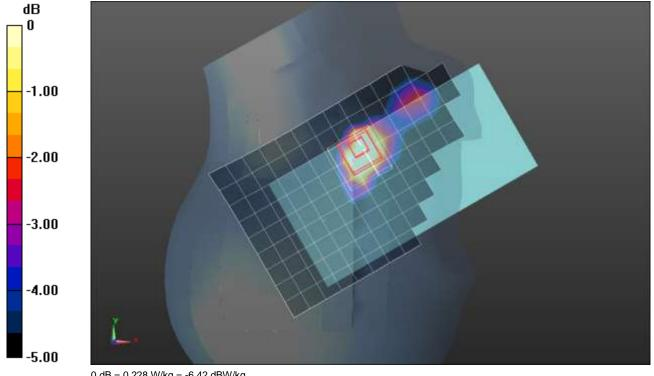
Frequency: 3560 MHz; Duty Cycle: 1:1.59956; Room Ambient Temperature: 24.0°C; Liquid Temperature: 23.0°C Medium parameters used: f = 3560 MHz;  $\sigma = 2.829$  S/m;  $\varepsilon_r = 38.091$ ;  $\rho = 1000$  kg/m<sup>3</sup> Dasy Configuration:
