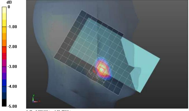
Frequency: 2310 MHz; Duty Cycle: 1:1; Room Ambient Temperature: 24.0°C; Liquid Temperature: 23.0°C Medium parameters used: f = 2310 MHz;  $\sigma = 1.744$  S/m;  $\varepsilon_r = 37.901$ ;  $\rho = 1000$  kg/m<sup>3</sup> Dasy Configuration:
