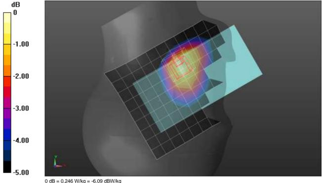
Frequency: 782 MHz; Duty Cycle: 1:1; Room Ambient Temperature: 24.0°C; Liquid Temperature: 23.0°C Medium parameters used (interpolated): f = 782 MHz;  $\sigma = 0.892$  S/m;  $\epsilon_r = 41.267$ ;  $\rho = 1000$  kg/m³ Dasy Configuration:
