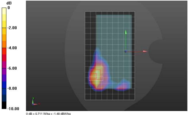
Frequency: 2593 MHz; Duty Cycle: 1:1; Room Ambient Temperature: 24.0°C; Liquid Temperature: 23.0°C Medium parameters used (interpolated): f = 2593 MHz;  $\sigma = 1.921$  S/m;  $\epsilon_r = 37.642$ ;  $\rho = 1000$  kg/m³ Dasy Configuration:
