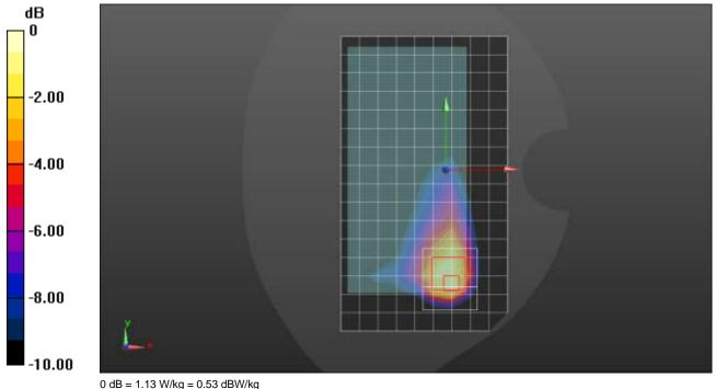
Frequency: 2535 MHz; Duty Cycle: 1:1; Room Ambient Temperature: 24.0°C; Liquid Temperature: 23.0°C Medium parameters used: f = 2535 MHz;  $\sigma$  = 1.918 S/m;  $\epsilon_r$  = 38.906;  $\rho$  = 1000 kg/m³ Dasy Configuration:
