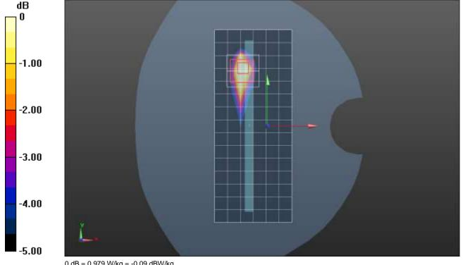
Frequency: 3560 MHz; Duty Cycle: 1:1.59956; Room Ambient Temperature: 24.0°C; Liquid Temperature: 23.0°C Medium parameters used: f = 3560 MHz;  $\sigma = 2.839$  S/m;  $\varepsilon_r = 38.281$ ;  $\rho = 1000$  kg/m<sup>3</sup> Dasy Configuration:
