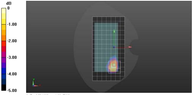
Frequency: 1860 MHz; Duty Cycle: 1:1; Room Ambient Temperature: 24.0°C; Liquid Temperature: 23.0°C Medium parameters used: f = 1860 MHz;  $\sigma = 1.418$  S/m;  $\epsilon_r = 38.452$ ;  $\rho = 1000$  kg/m³ Dasy Configuration:
