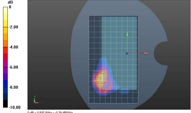
Frequency: 2310 MHz; Duty Cycle: 1:1; Room Ambient Temperature: 24.0°C; Liquid Temperature: 23.0°C Medium parameters used: f = 2310 MHz;  $\sigma = 1.619 \text{ S/m}$ ;  $\varepsilon_r = 37.634$ ;  $\rho = 1000 \text{ kg/m}^3$ Dasy Configuration:
