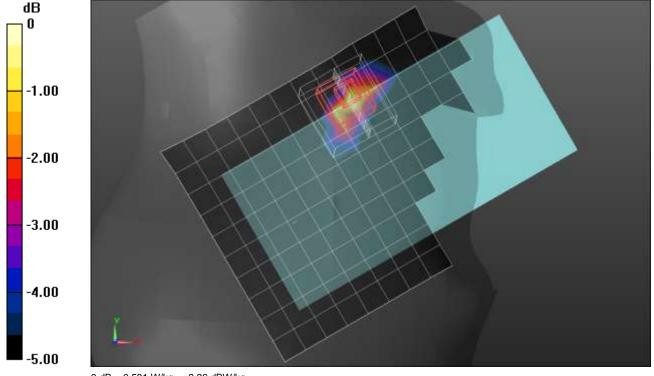
Frequency: 2535 MHz; Duty Cycle: 1:1; Room Ambient Temperature: 24.0°C; Liquid Temperature: 23.0°C Medium parameters used: f = 2535 MHz;  $\sigma$  = 1.852 S/m;  $\varepsilon_r$  = 38.337;  $\rho$  = 1000 kg/m<sup>3</sup> Dasy Configuration:
