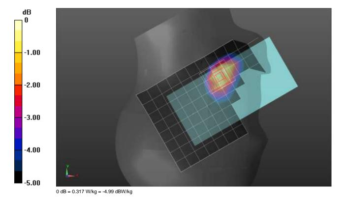
Frequency: 1745 MHz; Duty Cycle: 1:1; Room Ambient Temperature: 24.0°C; Liquid Temperature: 23.0°C Medium parameters used: f = 1745 MHz;  $\sigma = 1.387 \text{ S/m}$ ;  $\varepsilon_r = 38.733$ ;  $\rho = 1000 \text{ kg/m}^3$ Dasy Configuration:
