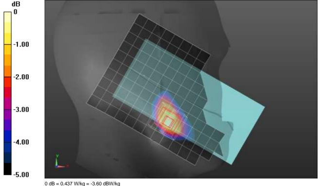
Frequency: 2535 MHz; Duty Cycle: 1:1; Room Ambient Temperature: 24.0°C; Liquid Temperature: 23.0°C Medium parameters used: f = 2535 MHz;  $\sigma = 1.892$  S/m;  $\varepsilon_r = 37.731$ ;  $\rho = 1000$  kg/m<sup>3</sup> Dasy Configuration:
