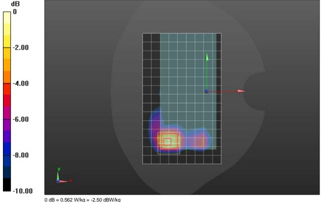
Frequency: 3499.98 MHz; Duty Cycle: 1:1; Room Ambient Temperature: 24.0°C; Liquid Temperature: 23.0°C Medium parameters used: f = 3500 MHz;  $\sigma = 2.817$  S/m;  $\epsilon_r = 39.478$ ;  $\rho = 1000$  kg/m³ Dasy Configuration:
