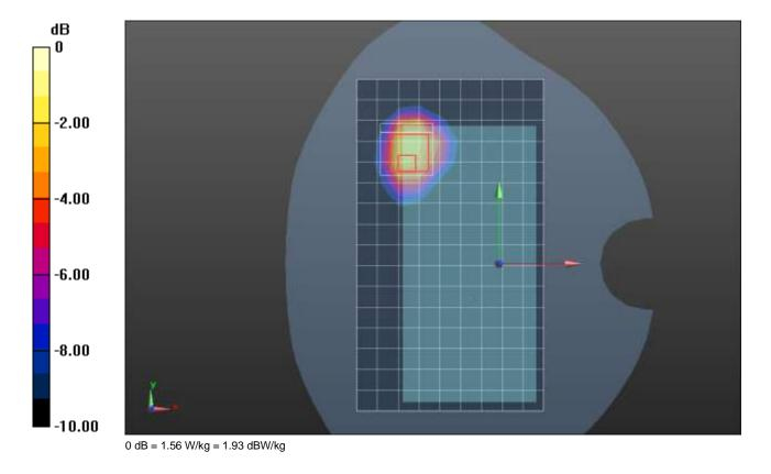
Frequency: 2593 MHz; Duty Cycle: 1:1.59956; Room Ambient Temperature: 24.0°C; Liquid Temperature: 23.0°C Medium parameters used (interpolated): f = 2593 MHz;  $\sigma$  = 1.938 S/m;  $\epsilon_r$  = 39.967;  $\rho$  = 1000 kg/m³ Dasy Configuration:
