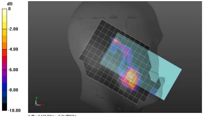
Frequency: 3840 MHz; Duty Cycle: 1:1; Room Ambient Temperature: 24.0°C; Liquid Temperature: 23.0°C Medium parameters used: f = 3840 MHz;  $\sigma = 3.143 \text{ S/m}$ ;  $\varepsilon_r = 38.909$ ;  $\rho = 1000 \text{ kg/m}^3$ Dasy Configuration:
