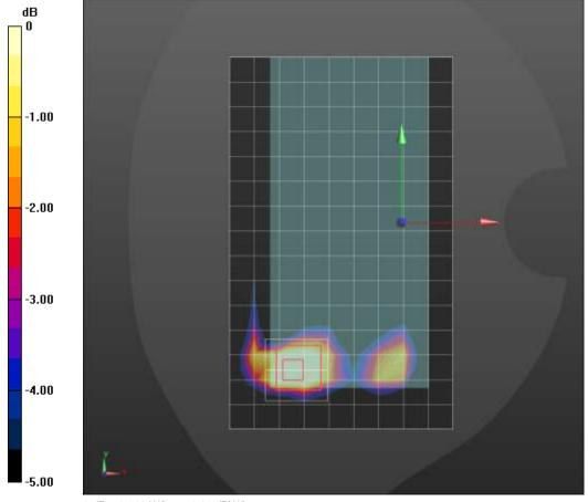
Frequency: 3560 MHz; Duty Cycle: 1:1.59956; Room Ambient Temperature: 24.0°C; Liquid Temperature: 23.0°C Medium parameters used: f = 3560 MHz;  $\sigma$  = 2.85 S/m;  $\epsilon_r$  = 39.428;  $\rho$  = 1000 kg/m<sup>3</sup> Dasy Configuration:
