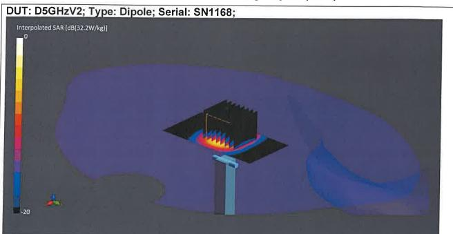
Communication System: CW UID: 0; Frequency: 5750.0 MHz; Duty Cycle: 1; Medium: HSL; Site65\_24Nov2021\_001812\_Head - 5GHz 5%; Medium parameters used: f = 5750.0 MHz;  $\sigma$  = 5.23 S/m;  $\epsilon_r$  = 34.9;  $\rho$  = 1000 kg/m3;  $\Delta \epsilon_r$  = -1.43 %;  $\Delta \sigma$  = 0.30 %; No correction Phantom section: Flat;
