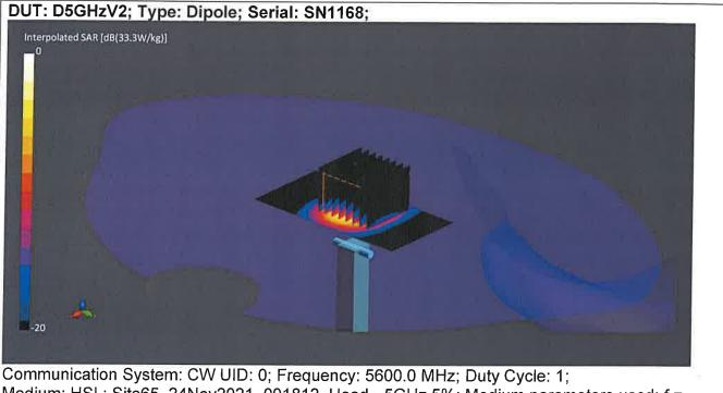
Medium: HSL; Site65\_24Nov2021\_001812\_Head - 5GHz 5%; Medium parameters used: f = 5600.0 MHz;  $\sigma$  = 5.06 S/m;  $\epsilon_r$  = 35.1;  $\rho$  = 1000 kg/m3;  $\Delta \epsilon_r$  = -1.07 %;  $\Delta \sigma$  = -0.10 %; No correction Phantom section: Flat;
