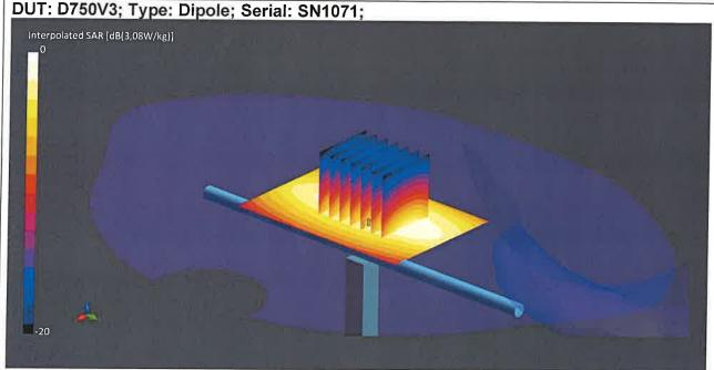
Communication System: CW UID: 0; Frequency: 750.0 MHz; Duty Cycle: 1; Medium: HSL; Site65\_23Nov2021\_030728\_Head - 750 900 1800 1900 5GHz 5%; Medium parameters used: f = 750.0 MHz;  $\sigma$  = 0.9 S/m;  $\epsilon_r$  = 42.3;  $\rho$  = 1000 kg/m3;  $\Delta\epsilon_r$  = 0.85 %;  $\Delta\sigma$  = 0.62 %; No correction
