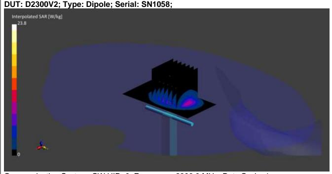
Communication System: CW UID: 0; Frequency: 2300.0 MHz; Duty Cycle: 1; Medium: HSL; Site65\_28Sep2021\_082639\_Head - 900 1800 1900 2300 2600 5%; Medium parameters used: f = 2300.0 MHz;  $\sigma$  = 1.71 S/m;  $\epsilon_r$  = 39.6;  $\rho$  = 1000 kg/m3;  $\Delta\epsilon_r$  = 0.38 %;  $\Delta\sigma$  = 2.71 %; No correction
