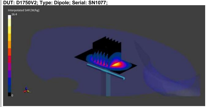
Communication System: CW UID: 0; Frequency: 1750.0 MHz; Duty Cycle: 1; Medium: HSL; Site65\_28Sep2021\_082639\_Head - 900 1800 1900 2300 2600 5%; Medium parameters used: f = 1750.0 MHz;  $\sigma$  = 1.35 S/m;  $\epsilon_r$  = 40.4;  $\rho$  = 1000 kg/m3;  $\Delta\epsilon_r$  = 0.91 %;  $\Delta\sigma$  = -1.51 %; No correction
