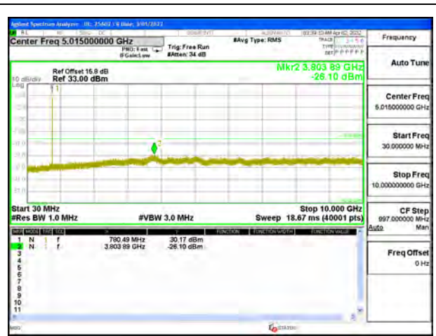
LTE B13 10MHz QPSK Middle Channel RB1-0
