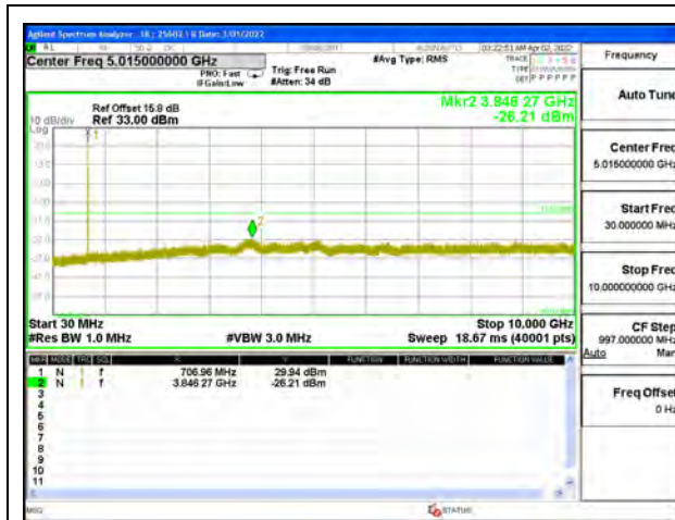
LTE B12 3MHz QPSK Middle Channel RB1-0
