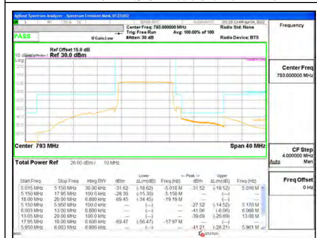
LTE B14 10MHz QPSK Middle Channel RB50-0
