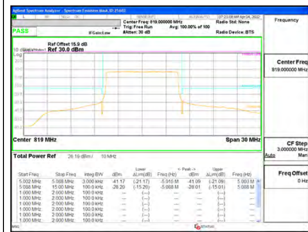
LTE B26 10MHz QPSK Middle Channel RB50-0
