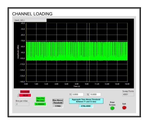
The level of traffic loading on the channel by the EUT is 47.86%
