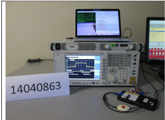
RF ANTENNA PORT CONDUCTED
