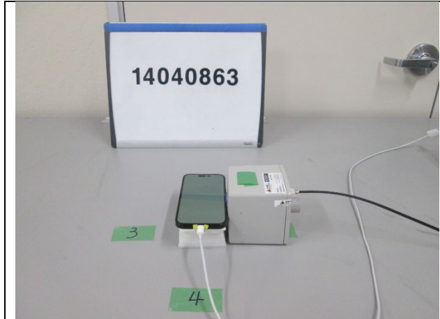
S1, RF Exposure Setup Photo
