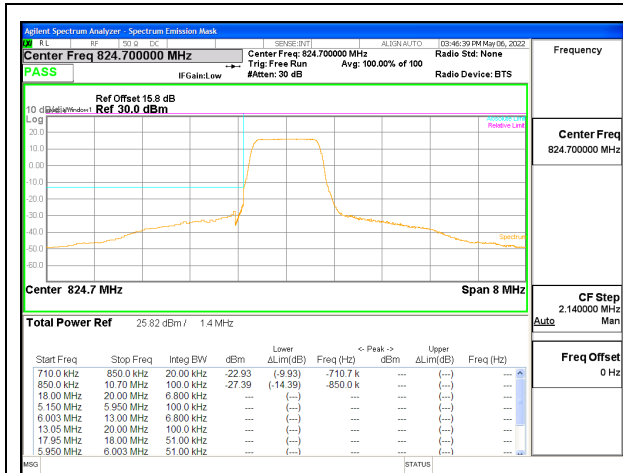
LTE B26 1.4MHz QPSK Low Channel RB6-0
