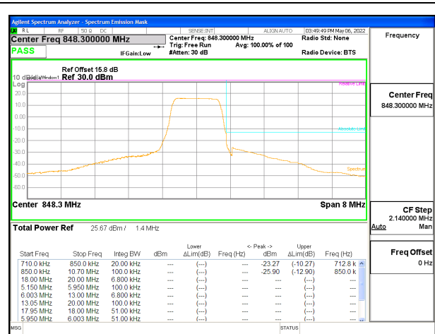
LTE B26 1.4MHz QPSK High Channel RB6-0
