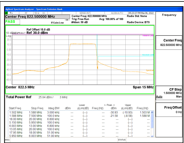
LTE B26 3MHz QPSK High Channel RB15-0
