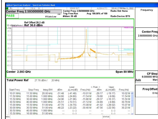
LTE B41 20MHz QPSK Middle Channel RB1-99
