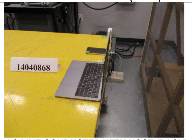
AC LINE CONDUCTED WITH HOST (BACK)
