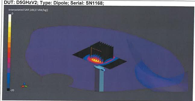
Communication System: CW UID: 0; Frequency: 5250.0 MHz; Duty Cycle: 1; Medium: HSL; Site65\_24Nov2021\_001812\_Head - 5GHz 5%; Medium parameters used: f = 5250.0 MHz;  $\sigma$  = 4.66 S/m;  $\epsilon_r$  = 35.8;  $\rho$  = 1000 kg/m3;  $\Delta\epsilon_r$  = -0.28 %;  $\Delta\sigma$  = -1.02 %; No correction Phantom section: Flat:
