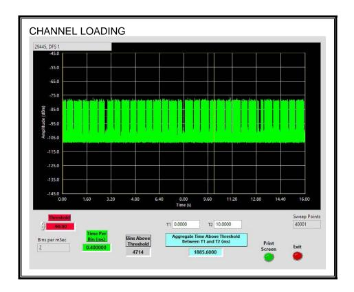
The level of traffic loading on the channel by the EUT is 18.85%
