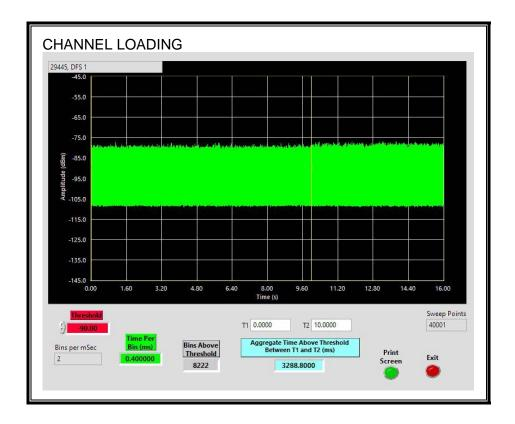
The level of traffic loading on the channel by the EUT is 32.88%
