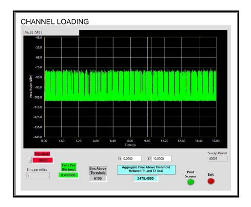
The level of traffic loading on the channel by the EUT is 24.78%
