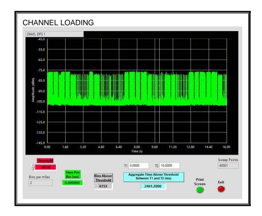
The level of traffic loading on the channel by the EUT is 24.61%
