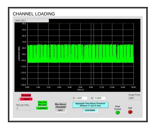
The level of traffic loading on the channel by the EUT is 22.68%
