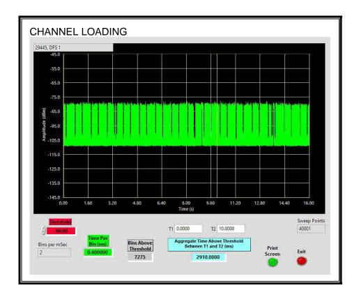
The level of traffic loading on the channel by the EUT is 29.1%
