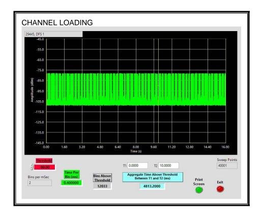
The level of traffic loading on the channel by the EUT is 48.13%
