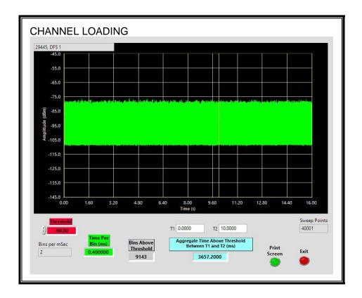
The level of traffic loading on the channel by the EUT is 36.57%
