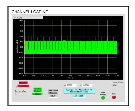
The level of traffic loading on the channel by the Peer Slave is 22.51%
