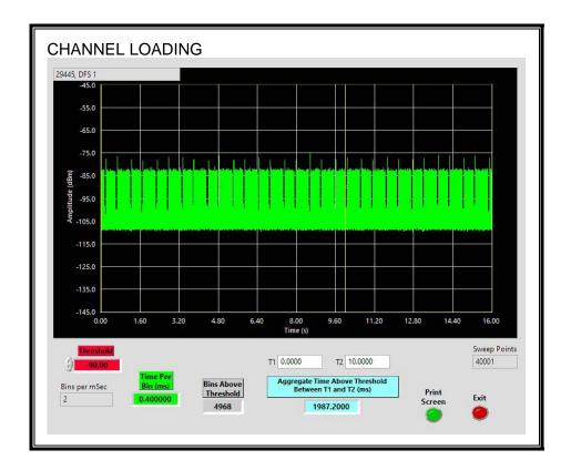
The level of traffic loading on the channel by the Peer Slave is 19.87%
