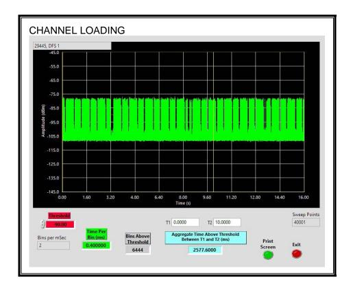
The level of traffic loading on the channel by the EUT is 25.77%
