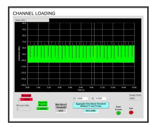
The level of traffic loading on the channel by the Peer Slave is 18.13%
