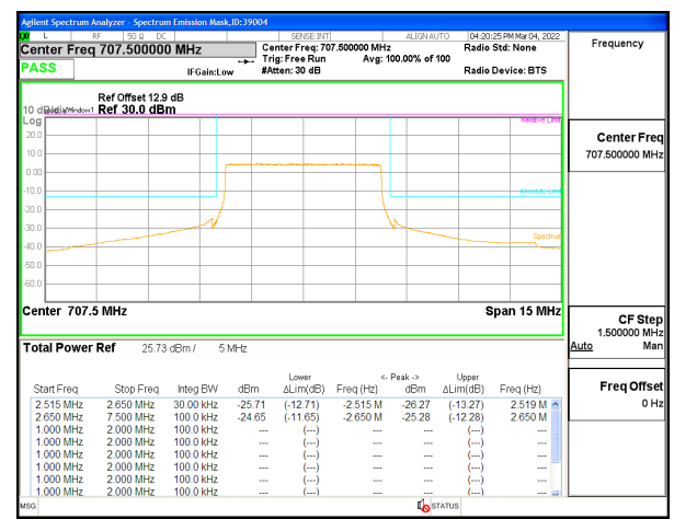
LTE B12 5MHz QPSK Middle Channel RB25-0
