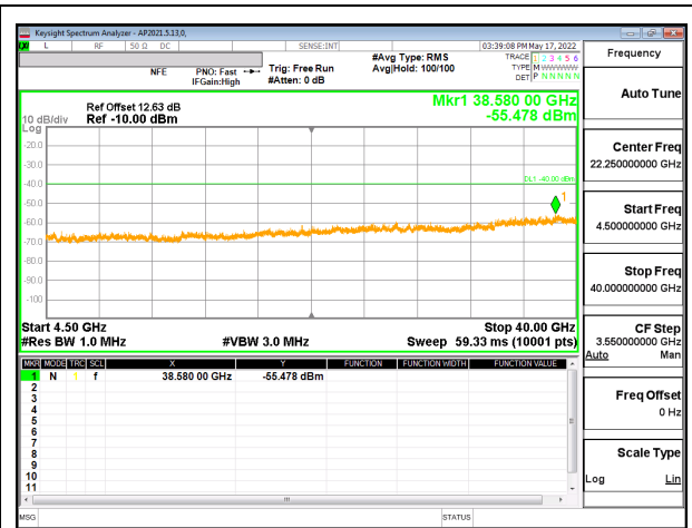
5G NR n48 40MHz BPSK High Channel RB1-105 (4.5G to 40G) , ID:52275
