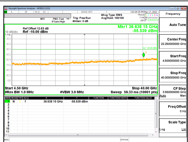
5G NR n48 30MHz BPSK High Channel RB1-1 (4.5G to 40G) , ID:52275
