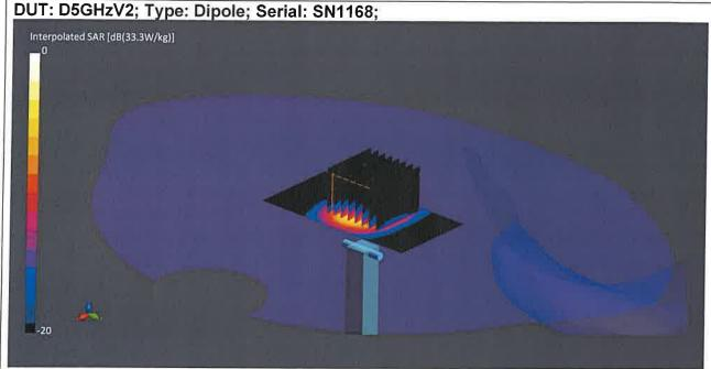
Communication System: CW UID: 0; Frequency: 5600.0 MHz; Duty Cycle: 1; Medium: HSL; Site65\_24Nov2021\_001812\_Head - 5GHz 5%; Medium parameters used: f = 5600.0 MHz;  $\sigma$  = 5.06 S/m;  $\epsilon_r$  = 35.1;  $\rho$  = 1000 kg/m3;  $\Delta \epsilon_r$  = -1.07 %;  $\Delta \sigma$  = -0.10 %; No correction Phantom section: Flat:
