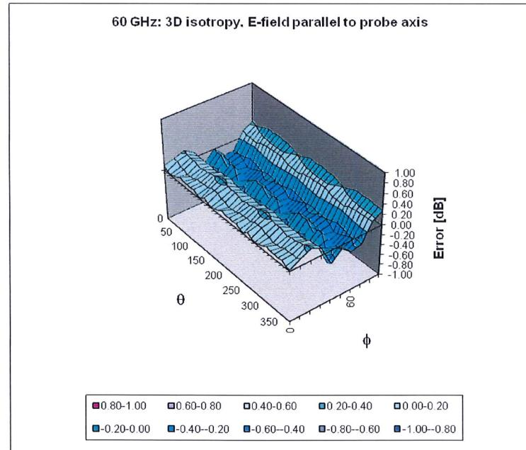
Probe isotropy for  $E_{\text{tot}}$ : probe rotated  $\phi = 0^\circ$  to  $360^\circ$ , tilted from field propagation direction  $\vec{k}$
