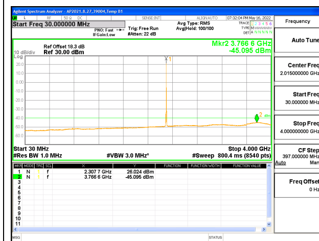
LTE B30 5MHz QPSK Mid Channel RB1-0 (30MHz to 4GHz)
