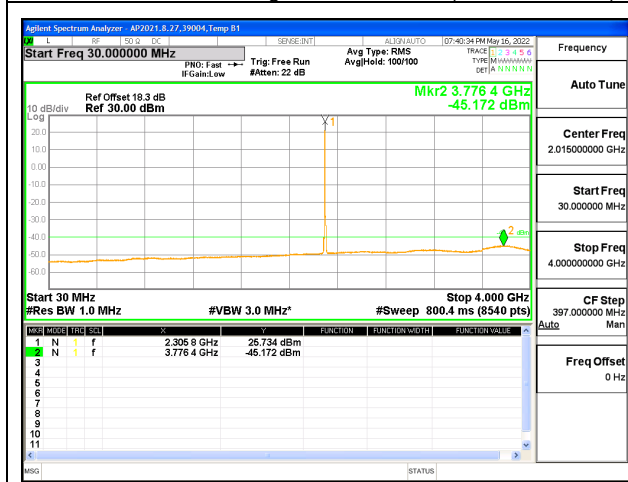
LTE B30 10MHz QPSK Mid Channel RB1-0 (30MHz to 4GHz)
