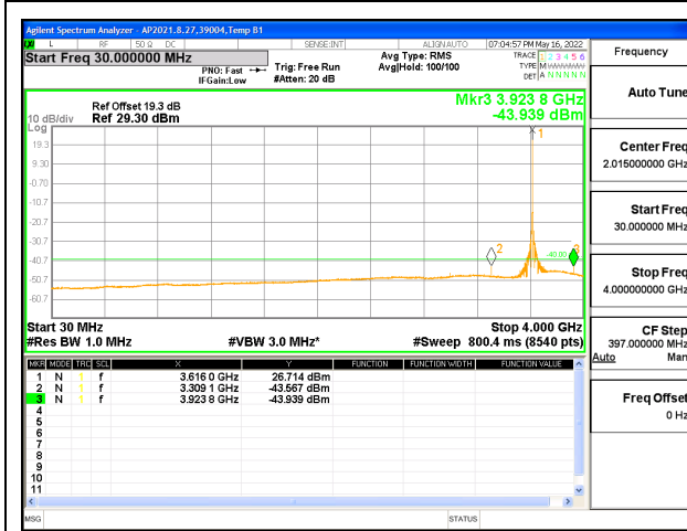
LTE B48 20MHz QPSK Mid Channel RB1-0 (30MHz to 4GHz)
