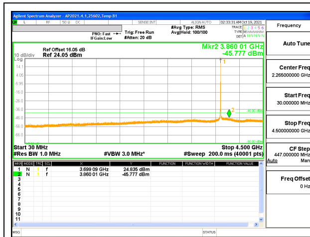
5G NR n48 10MHz BPSK High Channel RB1-23 (30M to 4.5G)
