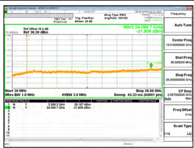
5G NR n7 20MHz BPSK High Channel RB1-105
