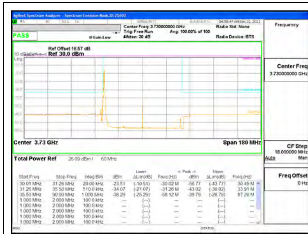
5G NR n77 60MHz BPSK Low Channel RB1-0
