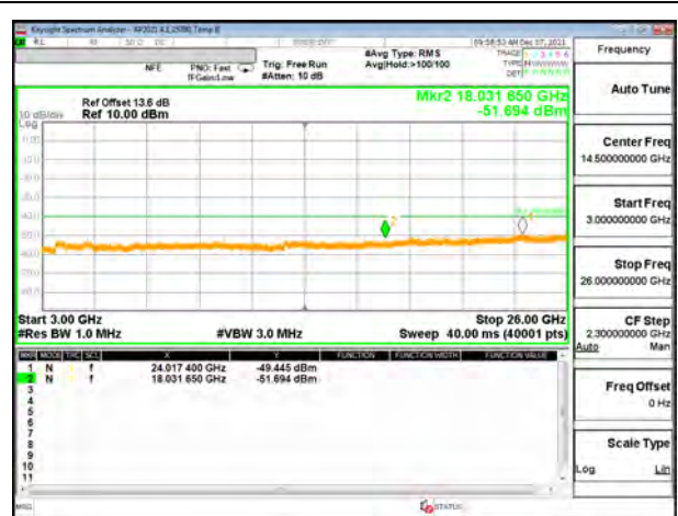
5G NR n30 5MHz BPSK Low Channel RB1-0 (3G to 26G)
