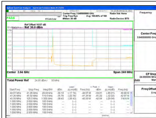
5G NR n77 80MHz BPSK High Channel RB1-0
