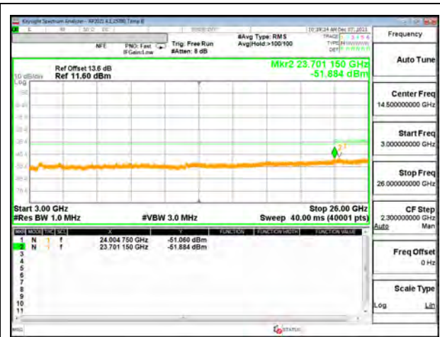
5G NR n30 10MHz BPSK Mid Channel RB1-1 (3G to 26G)
