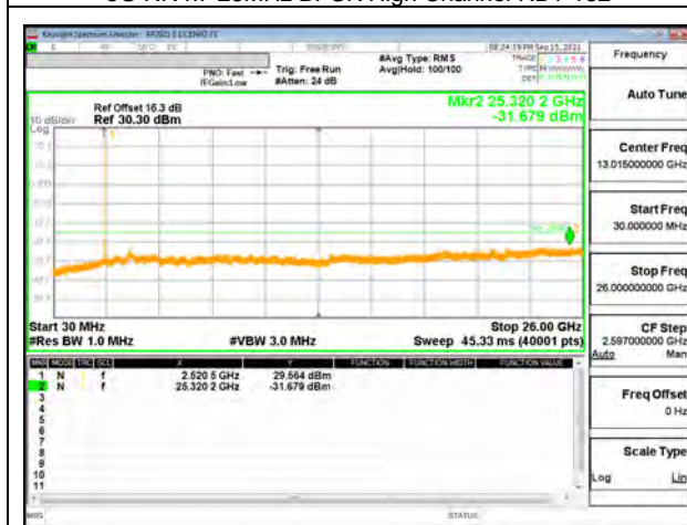
5G NR n7 30MHz BPSK Middle Channel RB1-1
