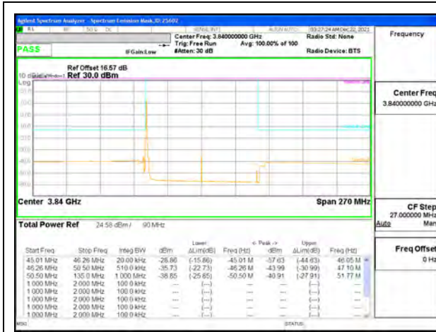
5G NR n77 90MHz BPSK Middle Channel RB1-0
