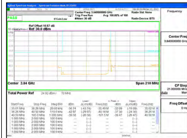
5G NR n77 70MHz BPSK Middle Channel RB1-188
