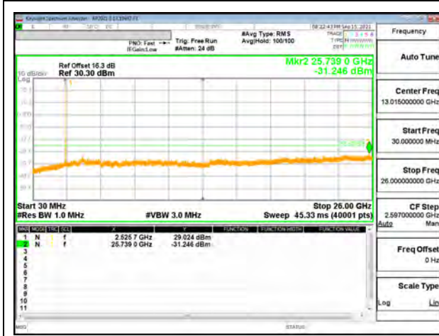
5G NR n7 20MHz BPSK Middle Channel RB1-1
