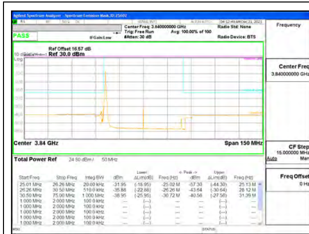
5G NR n77 50MHz BPSK Middle Channel RB1-0
