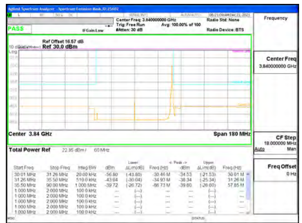
5G NR n77 60MHz BPSK Middle Channel RB1-161
