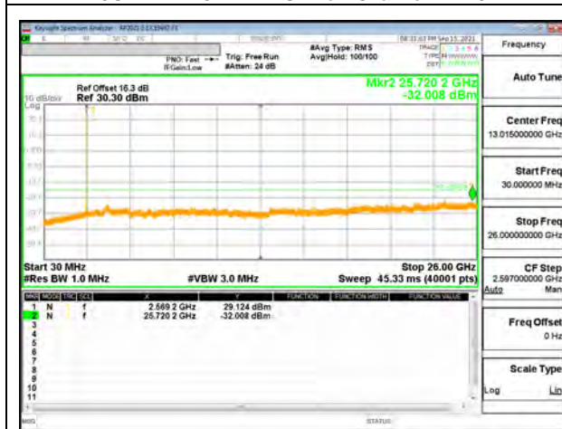
5G NR n7 25MHz BPSK High Channel RB1-132
