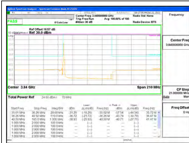
5G NR n77 70MHz BPSK Middle Channel RB1-0
