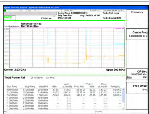
5G NR n77 100MHz BPSK High Channel RB1-272
