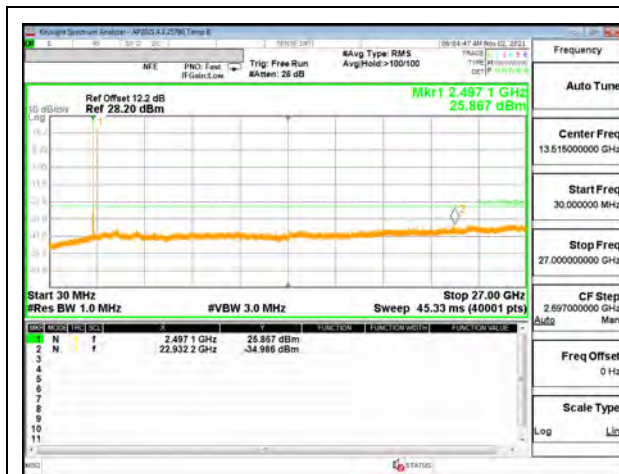
5G NR n41 40MHz BPSK Low Channel RB1-0
