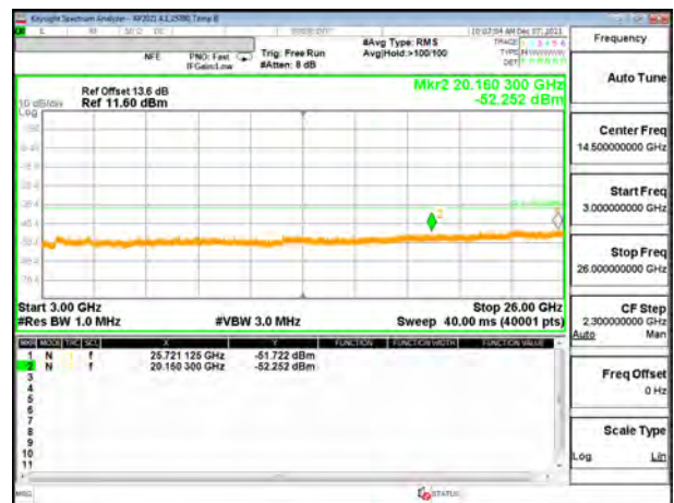
5G NR n30 5MHz BPSK Mid Channel RB1-1 (3G to 26G)
