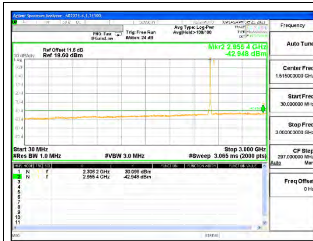
5G NR n30 10MHz BPSK Mid Channel RB1-1 (30M to 3G)
