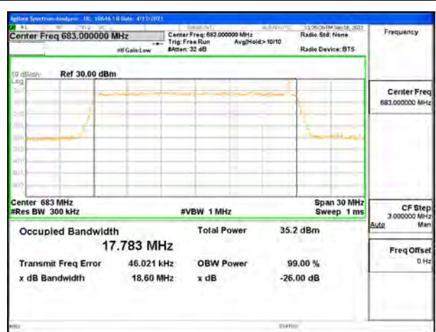
LTE B71 20MHz QPSK Middle Channel RB100-0
