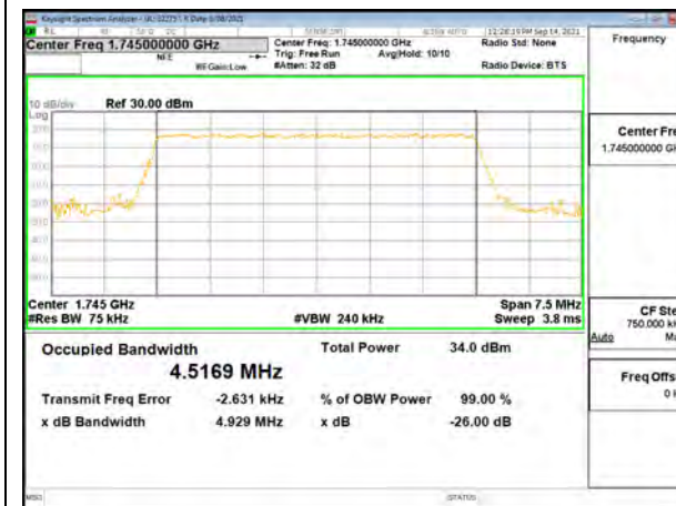
LTE B66 5MHz QPSK Middle Channel RB25-0
