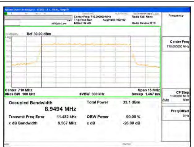
LTE B17 10MHz QPSK Middle Channel RB50-0
