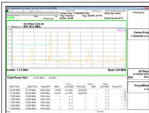
LTE B66C 20MHz + 20MHz 16QAM Low Ch RB1-0 + RB1-0
