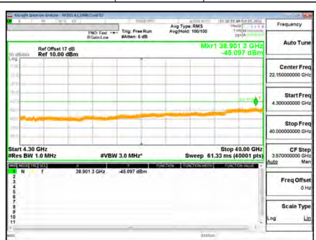
LTE B48 20MHz + 20MHz QPSK Middle Ch RB1-99 + RB1-0 (4.5GHz to 40GHz)
