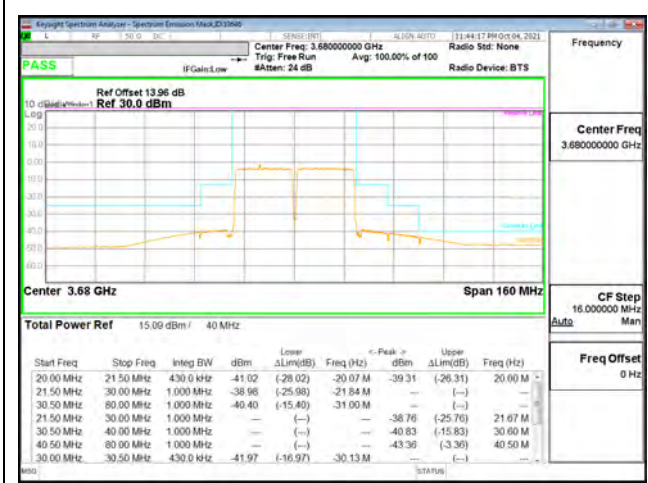
LTE B48 20MHz + 20MHz QPSK High Ch RB100-0 + RB100-0
