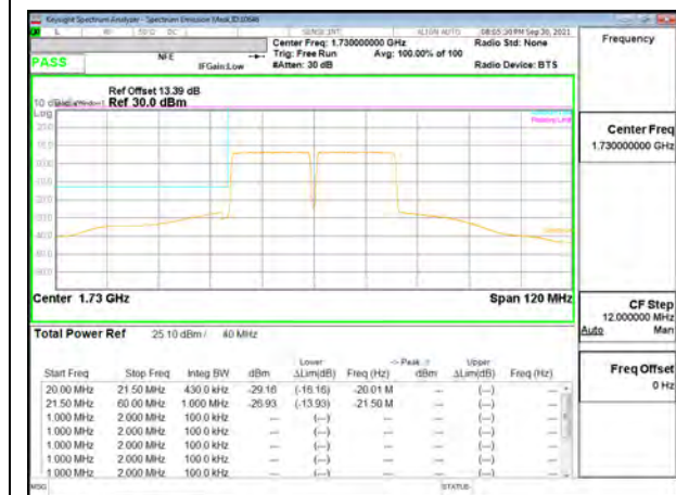
LTE B66C 20MHz + 20MHz QPSK Low Ch RB100-0 + RB100-0
