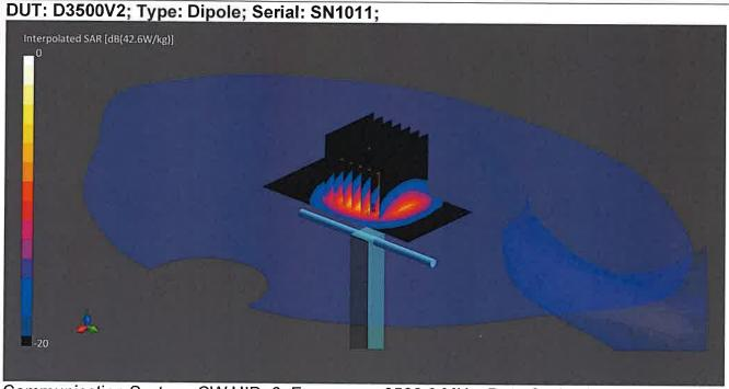
Communication System: CW UID: 0; Frequency: 3500.0 MHz; Duty Cycle: 1; Medium: HSL; Site65\_14Apr2021\_183123\_Head - 3500.5%; Medium parameters used: f = 3500.0 MHz;  $\sigma$  = 2.97 S/m;  $\epsilon_r$  = 37.3;  $\rho$  = 1000 kg/m3;  $\Delta\epsilon_r$  = -1.72 %;  $\Delta\sigma$  = 2.03 %; No correction Phantom section: Flat:
