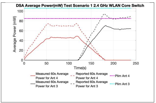
Figure 2 60 Second Average Power vs Time, 2.4GHz
