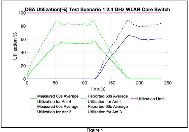
60 Second Aggregated SAR Utilization vs Time, 2.4GHz
