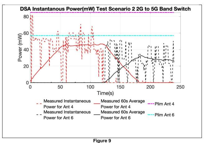
60 Second Average Power vs Time during Band Switch and Instantaneous Power
