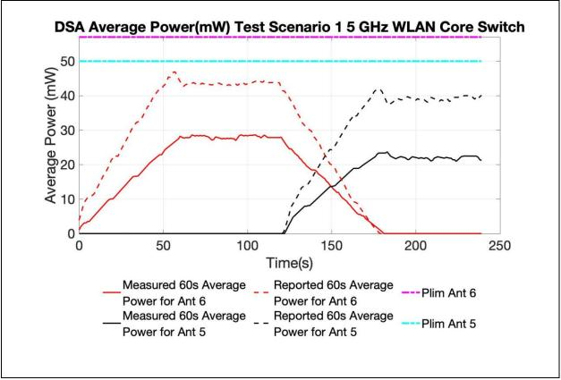
Figure 5 60 Second Average Power vs Time, 5GHz
