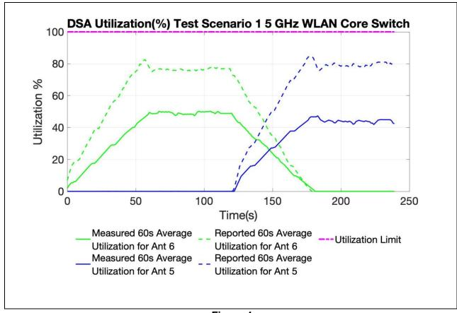
Figure 4 60 Second Aggregated SAR Utilization vs Time, 5GHz
