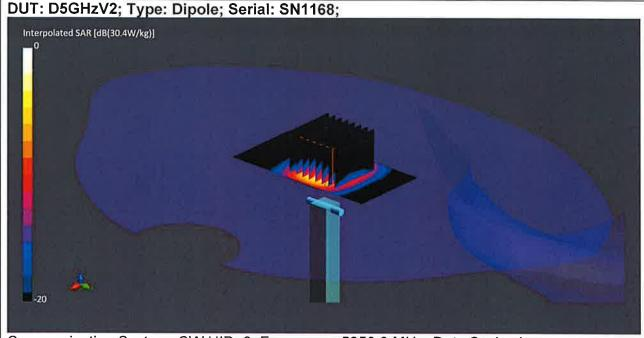
Communication System: CW UID: 0; Frequency: 5250.0 MHz; Duty Cycle: 1; Medium: HSL; Site65\_26Nov2020\_102813\_Head - 5Ghz 5%; Medium parameters used: f = 5250.0 MHz;  $\sigma$  = 4.69 S/m;  $\epsilon_r$  = 35.8;  $\rho$  = 1000 kg/m3;  $\Delta\epsilon_r$  = -0.44 %;  $\Delta\sigma$  = -0.42 %; No correction
