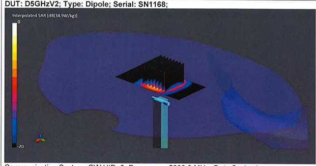
Communication System: CW UID: 0; Frequency: 5600.0 MHz; Duty Cycle: 1; Medium: HSL; Site65\_26Nov2020\_102813\_Head - 5Ghz 5%; Medium parameters used: f = 5600.0 MHz;  $\sigma$  = 5.07 S/m;  $\epsilon_r$  = 35.1;  $\rho$  = 1000 kg/m3;  $\Delta\epsilon_r$  = -1.22 %;  $\Delta\sigma$  = 0.14 %; No correction
