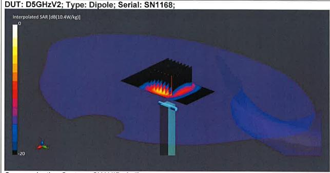
Communication System: CW UID: 0; Frequency: 5750.0 MHz; Duty Cycle: 1;
