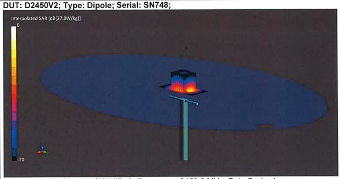
Communication System: CW UID: 0; Frequency: 2450.0 MHz; Duty Cycle: 1; Medium: HSL; Site59\_19Feb2021\_104323\_Head - 2450.5%; Medium parameters used: f = 2450.0 MHz;  $\sigma$  = 1.8 S/m;  $\epsilon_r$  = 39.6;  $\rho$  = 1000 kg/m3;  $\Delta \epsilon_r$  = 0.92 %;  $\Delta \sigma$  = 0.26 %; No correction Phantom section: Flat:
