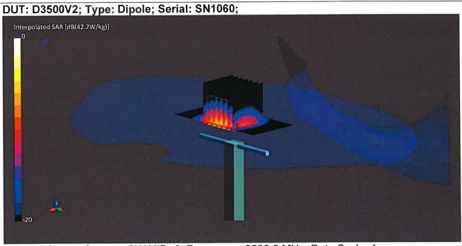
Communication System: CW UID: 0; Frequency: 3500.0 MHz; Duty Cycle: 1; Medium: HSL; Site59\_25Feb2021\_111544\_Head - 3500.5%; Medium parameters used: f = 3500.0 MHz;  $\sigma$  = 2.79 S/m;  $\epsilon_r$  = 39.4;  $\rho$  = 1000 kg/m3;  $\Delta \epsilon_r$  = 3.82 %;  $\Delta \sigma$  = -4.19 %; No correction Phantom section: Flat;
