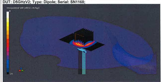
Communication System: CW UID: 0; Frequency: 5600.0 MHz; Duty Cycle: 1;
