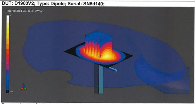
Communication System: CW UID: 0; Frequency: 1900.0 MHz; Duty Cycle: 1;
