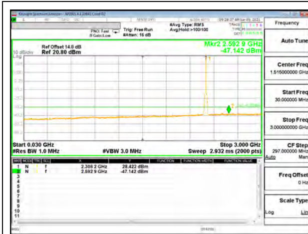
LTE 5G NR n30 5MHz BPSK Low Channel RB1-0 (30MHz to 3GHz)
