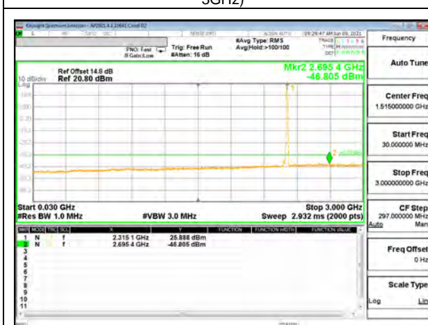
LTE 5G NR n30 5MHz BPSK High Channel RB1-24 (30MHz to 3GHz)
