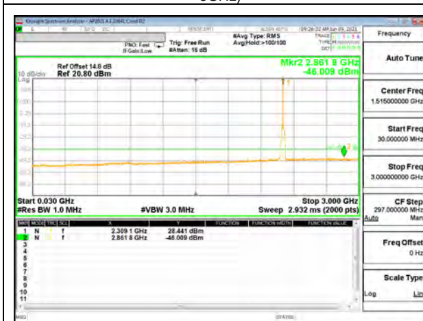
LTE 5G NR n30 5MHz BPSK Mid Channel RB1-1 (30MHz to 3GHz)
