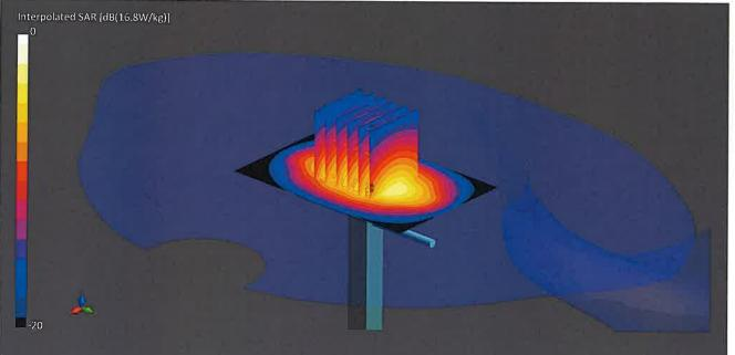
Communication System: CW UID: 0; Frequency: 1750.0 MHz; Duty Cycle: 1; Medium: HSL; Site65\_12Apr2021\_115940\_Head - 1750 1800 1900 2300 2450 2600 5%; Medium parameters used: f = 1750.0 MHz;  $\sigma$  = 1.35 S/m;  $\epsilon_r$  = 39.8;  $\rho$  = 1000 kg/m3;  $\Delta \epsilon_r$  = -0.62 %;  $\Delta \sigma$  = -1.80 %; No correction
