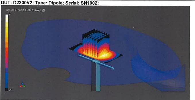
Communication System: CW UID: 0; Frequency: 2300.0 MHz; Duty Cycle: 1; Medium: HSL; Site65\_12Apr2021\_115940\_Head - 1750 1800 1900 2300 2450 2600 5%; Medium parameters used: f = 2300.0 MHz;  $\sigma$  = 1.7 S/m;  $\epsilon_r$  = 39;  $\rho$  = 1000 kg/m3;  $\Delta \epsilon_r$  = -1.19 %;  $\Delta \sigma$  = 2.28 %; No correction
