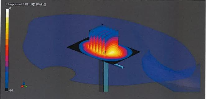
Communication System: CW UID: 0; Frequency: 1900.0 MHz; Duty Cycle: 1; Medium: HSL; Site65\_12Apr2021\_115940\_Head - 1750 1800 1900 2300 2450 2600 5%; Medium parameters used: f = 1900.0 MHz;  $\sigma$  = 1.44 S/m;  $\epsilon_r$  = 39.5;  $\rho$  = 1000 kg/m3;  $\Delta \epsilon_r$  = -1.17 %;  $\Delta \sigma$  = 2.77 %; No correction
