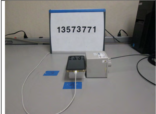
S1, RF Exposure Setup Photo
