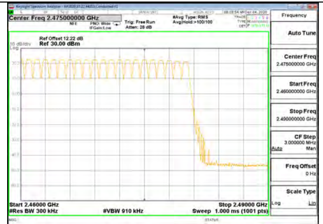
30MHz SPAN, SEGMENT 3 OF 3
