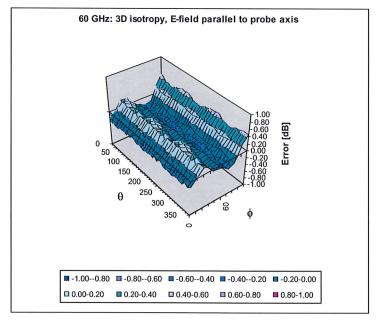
Probe isotropy for  $E_{tot}$ : probe rotated  $\phi$  = 0° to 360°, tilted from field propagation direction  $\vec{k}$  Parallel to the field propagation ( $\psi$  =0° - 90°) at 30 GHz: deviation within ± 0.40 dB Parallel to the field propagation ( $\psi$  =0° - 90°) at 60 GHz: deviation within ± 0.39 dB
