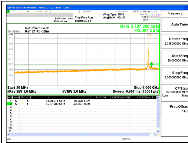
5G NR n48 20MHz BPSK High Channel RB1-50 (30MHz to 4GHz)
