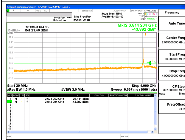
5G NR n48 10MHz BPSK Mid Channel RB1-1 (30MHz to 4GHz)
