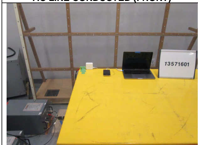
AC LINE CONDUCTED WITH HOST (FRONT)
