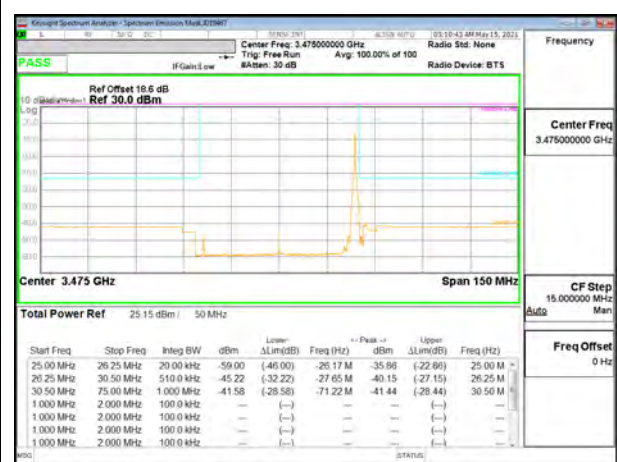
5G NR n77 50MHz BPSK Low Channel RB1-132
