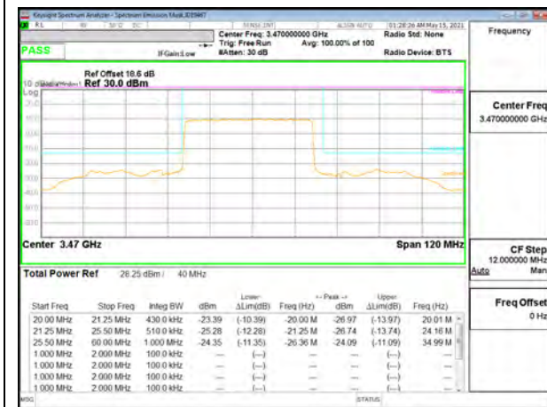
5G NR n77 40MHz BPSK Low Channel RB100-0
