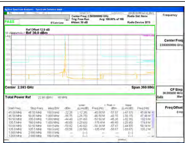
5G NR n41 90MHz BPSK Middle Channel RB1-0, ID 19467
