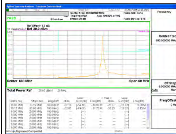
5G NR n71 20MHz BPSK Middle Channel RB1-105, ID 19467
