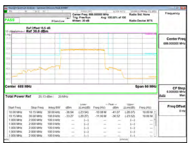
5G NR n71 20MHz BPSK High Channel RB100-0
