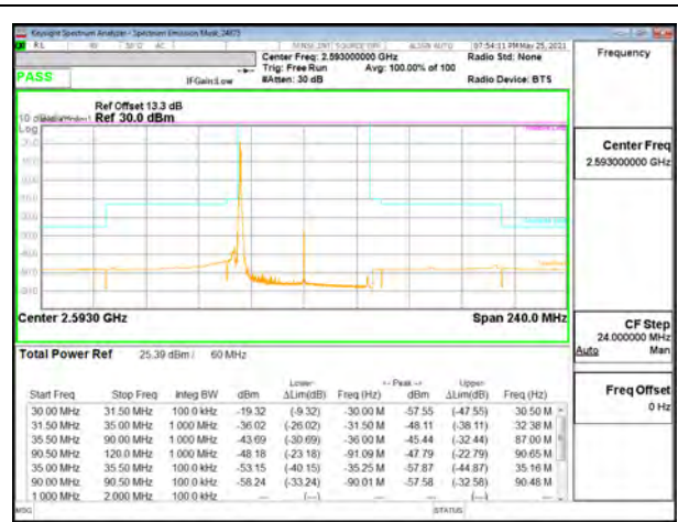
5G NR n41 60MHz BPSK Middle Channel RB1-0
