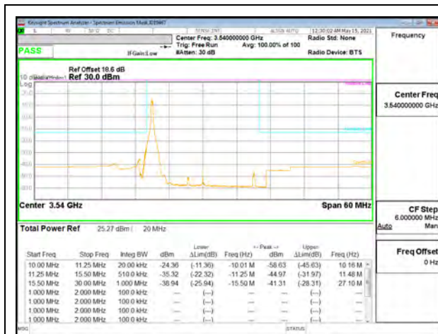
5G NR n77 20MHz BPSK High Channel RB1-0
