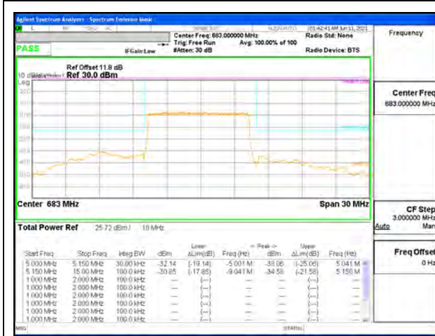
5G NR n71 10MHz BPSK Middle Channel RB50-0, ID 19467
