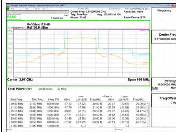
5G NR n41 40MHz BPSK High Channel RB100-0
