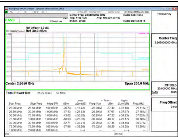
5G NR n41 50MHz BPSK High Channel RB1-0
