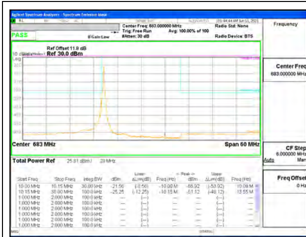
5G NR n71 20MHz BPSK Middle Channel RB1-0, ID 19467
