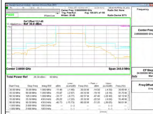
5G NR n41 60MHz BPSK High Channel RB162-0
