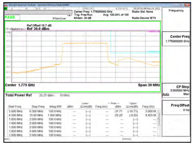
5G NR n66 10MHz BPSK High Channel RB50-0
