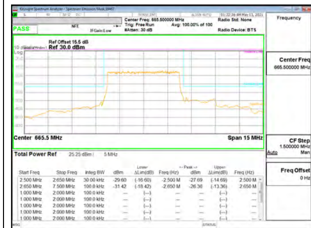
5G NR n71 5MHz BPSK Low Channel RB25-0
