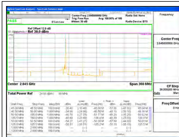
5G NR n41 90MHz BPSK High Channel RB1-0, ID 19467
