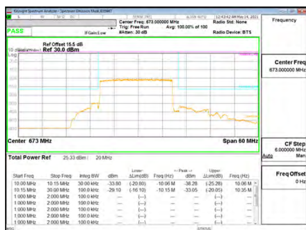
5G NR n71 20MHz BPSK Low Channel RB100-0
