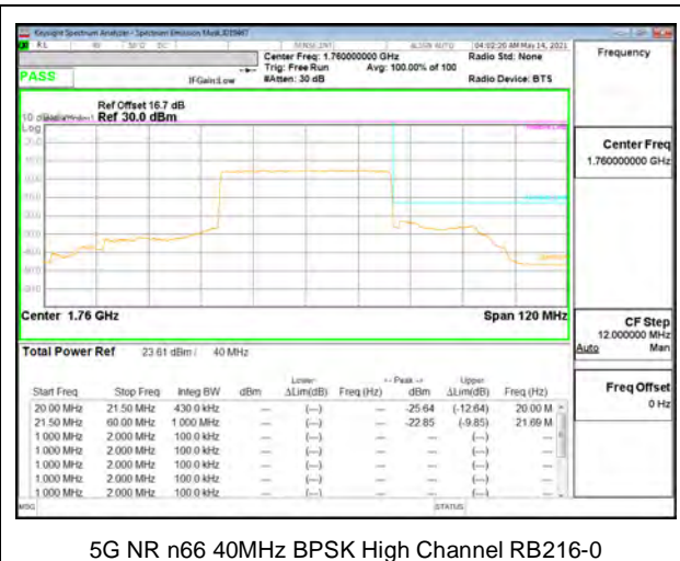
5G NR n66 40MHz BPSK High Channel RB216-0
