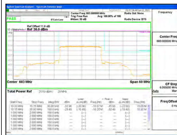
5G NR n71 20MHz BPSK Middle Channel RB100-0, ID 19467
