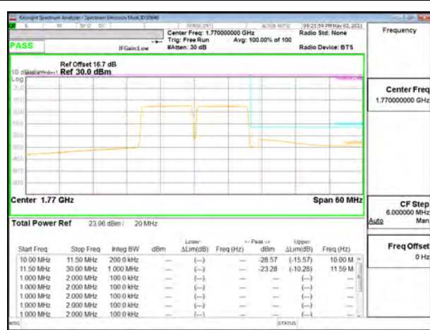
LTE B66B 10MHz + 10MHz QPSK High Ch RB50-0 + RB50-0
