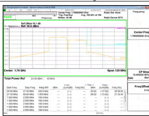
LTE B66C 20MHz + 20MHz 16QAM High Ch RB100-0 + RB100-0
