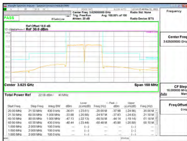
LTE B48 20MHz + 20MHz QPSK Mid Ch RB100-0 + RB100-0
