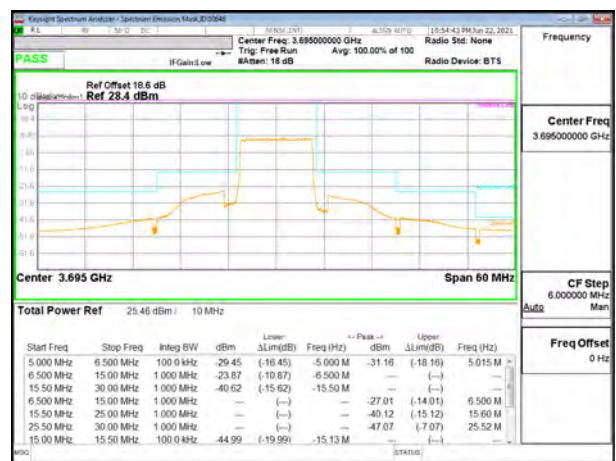
LTE B48 10MHz QPSK High Channel RB50-0
