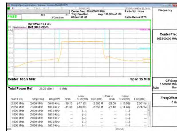
LTE B71 5MHz QPSK Low Channel RB25-0
