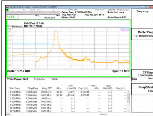
LTE B66 3MHz QPSK Low Channel RB1-0
