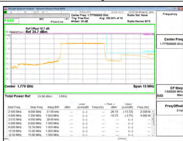
LTE B66 5MHz QPSK High Channel RB25-0
