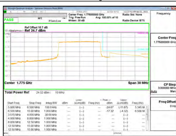
LTE B66 10MHz QPSK High Channel RB50-0
