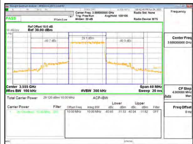
LTE B48 10MHz QPSK Low Channel RB50-0
