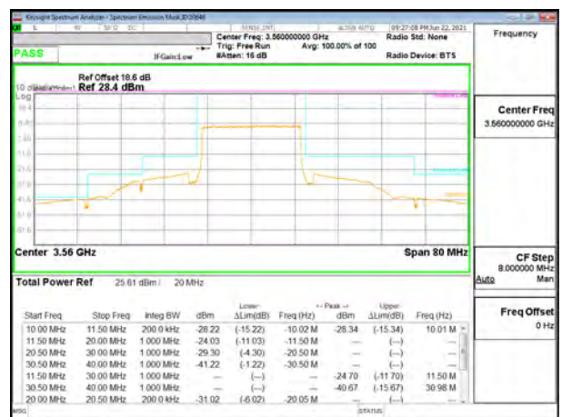
LTE B48 20MHz QPSK Low Channel RB100-0
