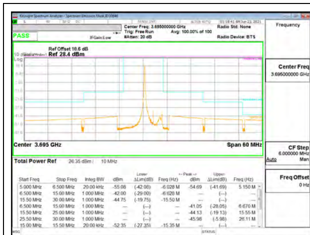
LTE B48 5MHz QPSK High Channel RB1-0
