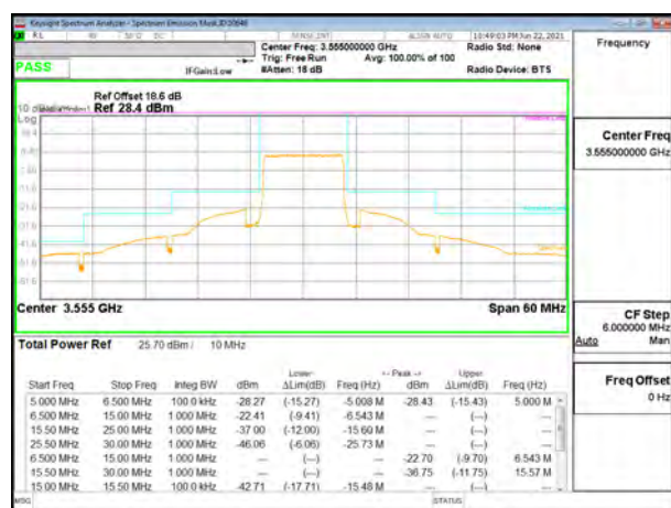
LTE B48 10MHz QPSK Low Channel RB50-0
