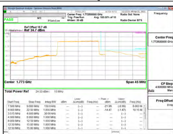
LTE B66 15MHz QPSK High Channel RB75-0
