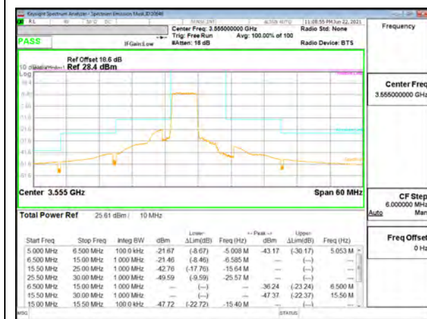
LTE B48 5MHz QPSK Low Channel RB25-0
