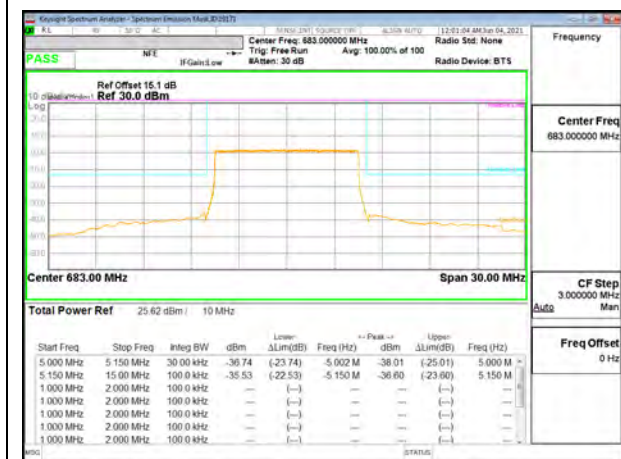
LTE B71 10MHz QPSK Middle Channel RB50-0
