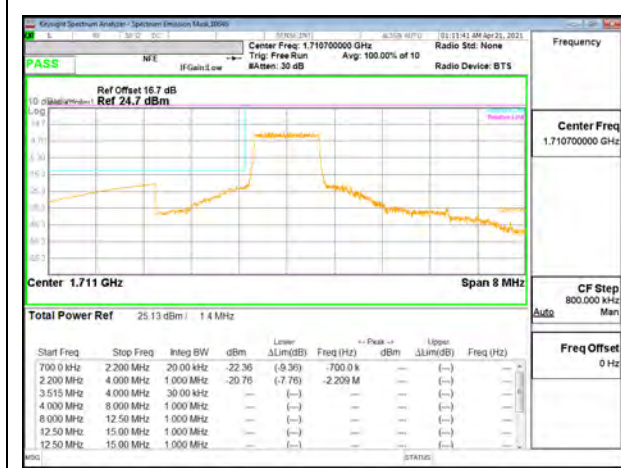
LTE B66 1.4MHz QPSK Low Channel RB6-0
