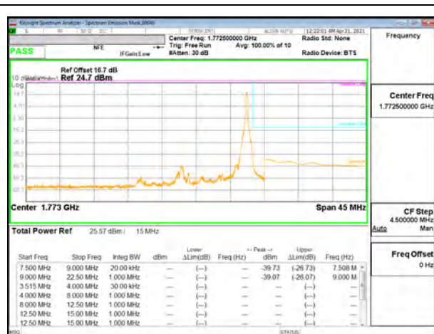
LTE B66 15MHz QPSK High Channel RB1-74
