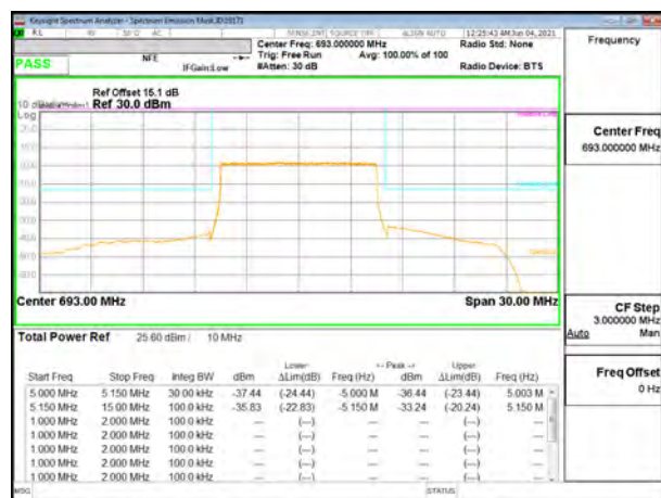
LTE B71 10MHz QPSK High Channel RB50-0
