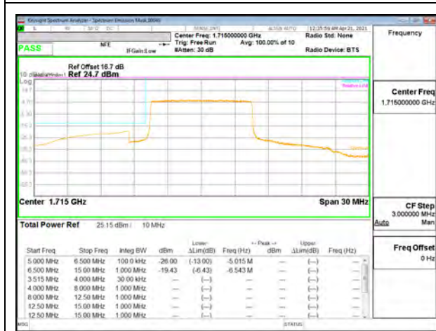
LTE B66 10MHz QPSK Low Channel RB50-0
