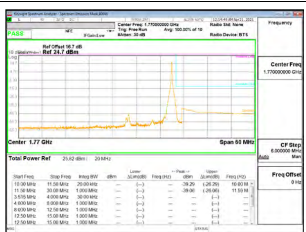
LTE B66 20MHz QPSK High Channel RB1-99
