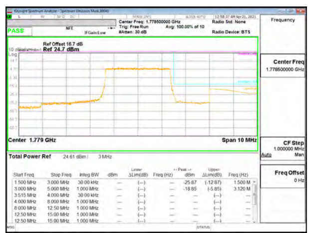
LTE B66 3MHz QPSK High Channel RB15-0
