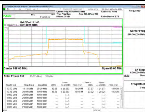
LTE B71 20MHz QPSK High Channel RB100-0
