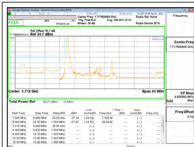
LTE B66 15MHz QPSK Low Channel RB1-0
