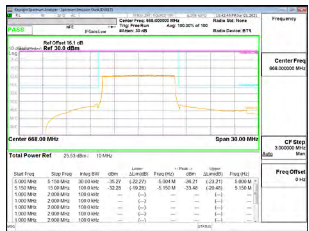
LTE B71 10MHz QPSK Low Channel RB50-0
