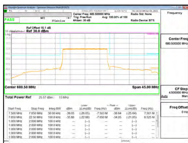
LTE B71 15MHz QPSK Middle Channel RB75-0
