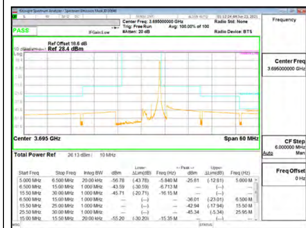
LTE B48 5MHz QPSK High Channel RB1-24
