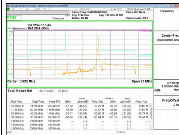
LTE B48 20MHz QPSK Middle Channel RB1-99
