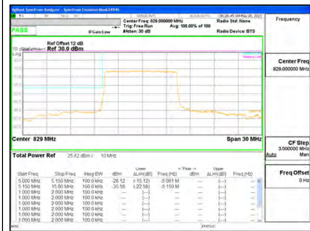
5G NR n5 10MHz BPSK Low Channel RB50-0
