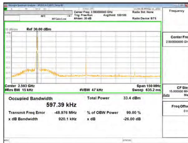
5G NR n41 100MHz BPSK Middle Channel RB1-0
