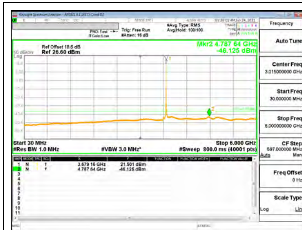
LTE B48 20MHz + 20MHz QPSK High Ch RB1-99 + RB1-0 (30MHz to 6GHz)
