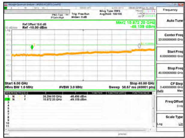
LTE B48 20MHz + 20MHz QPSK Middle Ch RB1-99 + RB1-0 (6GHz to 40GHz)
