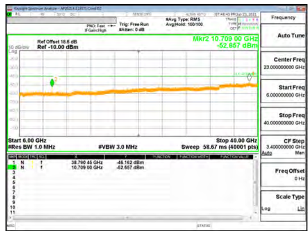
LTE B48 20MHz + 20MHz QPSK Low Ch RB1-99 + RB1-0 (6GHz to 40GHz)
