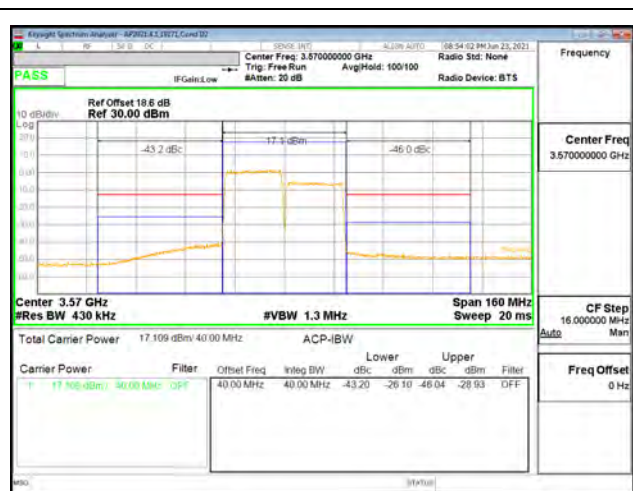
LTE B48 20MHz + 20MHz 16QAM Low Ch RB100-0 + RB100-0
