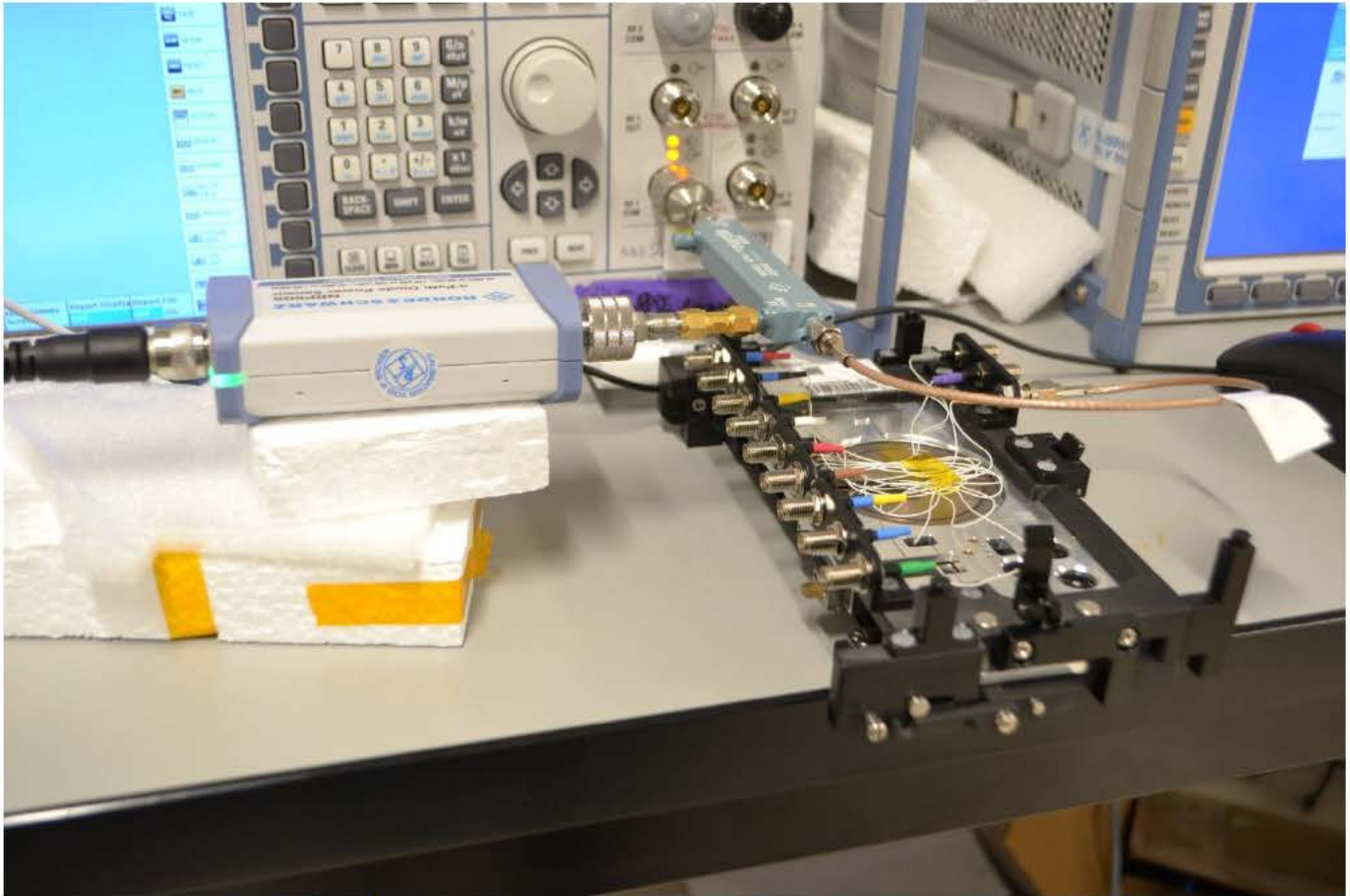
Figure C-1 CMW Conducted power test measurement setup single port
