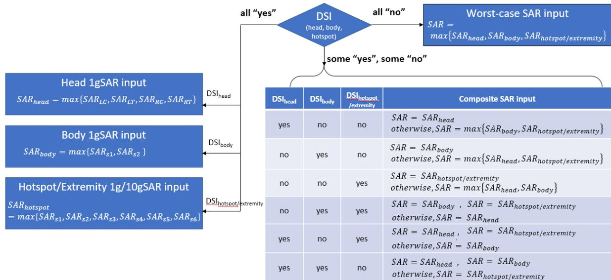
Figure 2-2: Worst-case SAR determination based on DSI
