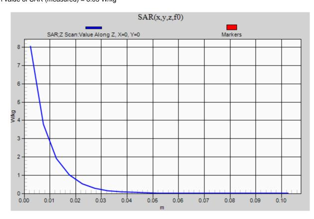
Frequency: 5600 MHz; Duty Cycle: 1:1; Room Ambient Temperature: 24.0°C; Liquid Temperature: 23.0°C Medium parameters used: f = 5600 MHz;  $\sigma$  = 5.023 S/m;  $\epsilon_r$  = 34.22;  $\rho$  = 1000 kg/m<sup>3</sup> DASY5 Configuration:
