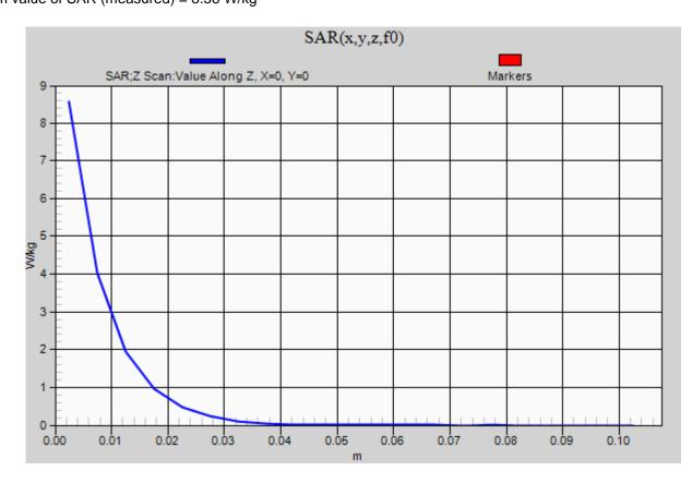
Frequency: 2450 MHz; Duty Cycle: 1:1; Room Ambient Temperature: 24.0°C; Liquid Temperature: 23.0°C Medium parameters used: f = 2450 MHz;  $\sigma$  = 1.862 S/m;  $\epsilon_r$  = 39.462;  $\rho$  = 1000 kg/m<sup>3</sup> DASY5 Configuration:
