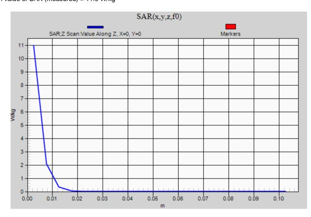
Frequency: 2600 MHz; Duty Cycle: 1:1; Room Ambient Temperature: 24.0°C; Liquid Temperature: 23.0°C Medium parameters used: f = 2600 MHz;  $\sigma$  = 1.96 S/m;  $\epsilon_r$  = 39.558;  $\rho$  = 1000 kg/m<sup>3</sup> DASY5 Configuration:
