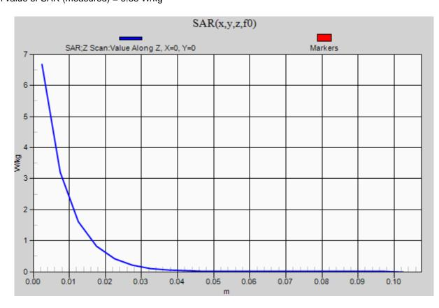
Frequency: 2600 MHz; Duty Cycle: 1:1; Room Ambient Temperature: 24.0°C; Liquid Temperature: 23.0°C Medium parameters used: f = 2600 MHz;  $\sigma$  = 1.945 S/m;  $\epsilon_r$  = 37.721;  $\rho$  = 1000 kg/m<sup>3</sup> DASY5 Configuration:
