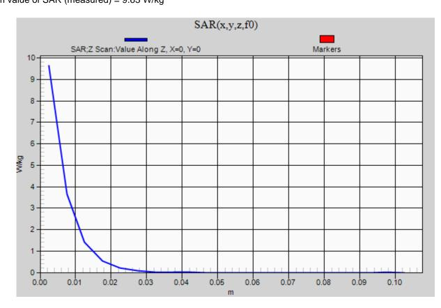
Frequency: 3700 MHz; Duty Cycle: 1:1; Room Ambient Temperature: 24.0°C; Liquid Temperature: 23.0°C Medium parameters used: f = 3700 MHz;  $\sigma$  = 3.028 S/m;  $\epsilon_r$  = 39.312;  $\rho$  = 1000 kg/m<sup>3</sup> DASY5 Configuration:
