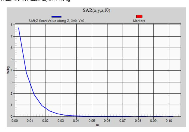
Frequency: 1750 MHz; Duty Cycle: 1:1; Room Ambient Temperature: 24.0°C; Liquid Temperature: 23.0°C Medium parameters used: f = 1750 MHz;  $\sigma$  = 1.362 S/m;  $\epsilon_r$  = 38.175;  $\rho$  = 1000 kg/m<sup>3</sup> DASY5 Configuration:
