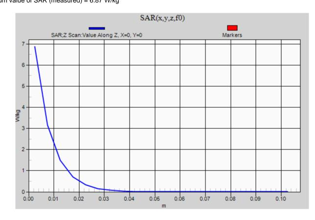
Frequency: 5250 MHz; Duty Cycle: 1:1; Room Ambient Temperature: 24.0°C; Liquid Temperature: 23.0°C Medium parameters used: f = 5250 MHz;  $\sigma$  = 4.642 S/m;  $\epsilon_r$  = 36.451;  $\rho$  = 1000 kg/m<sup>3</sup> DASY5 Configuration:
