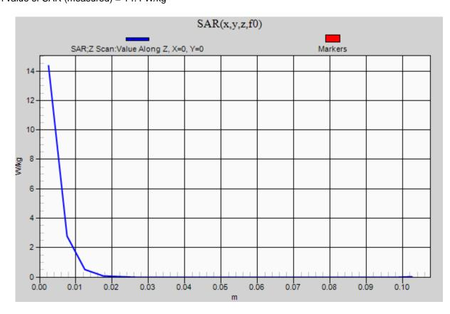
Frequency: 2600 MHz; Duty Cycle: 1:1; Room Ambient Temperature: 24.0°C; Liquid Temperature: 23.0°C Medium parameters used: f = 2600 MHz;  $\sigma$  = 1.943 S/m;  $\epsilon_r$  = 37.845;  $\rho$  = 1000 kg/m<sup>3</sup> DASY5 Configuration:
