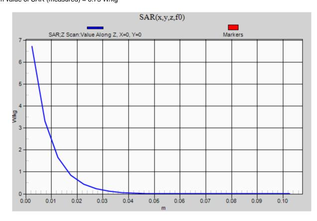
Frequency: 2450 MHz; Duty Cycle: 1:1; Room Ambient Temperature: 24.0°C; Liquid Temperature: 23.0°C Medium parameters used: f = 2450 MHz;  $\sigma$  = 1.863 S/m;  $\epsilon_r$  = 37.48;  $\rho$  = 1000 kg/m<sup>3</sup> DASY5 Configuration:
