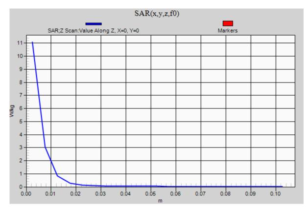
Frequency: 2300 MHz; Duty Cycle: 1:1; Room Ambient Temperature: 24.0°C; Liquid Temperature: 23.0°C Medium parameters used: f = 2300 MHz;  $\sigma$  = 1.713 S/m;  $\epsilon_r$  = 37.836;  $\rho$  = 1000 kg/m<sup>3</sup> DASY5 Configuration:
