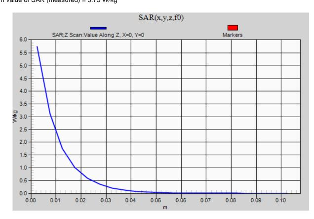
Frequency: 2600 MHz; Duty Cycle: 1:1; Room Ambient Temperature: 24.0°C; Liquid Temperature: 23.0°C Medium parameters used: f = 2600 MHz;  $\sigma$  = 1.955 S/m;  $\epsilon_r$  = 37.159;  $\rho$  = 1000 kg/m<sup>3</sup> DASY5 Configuration:
