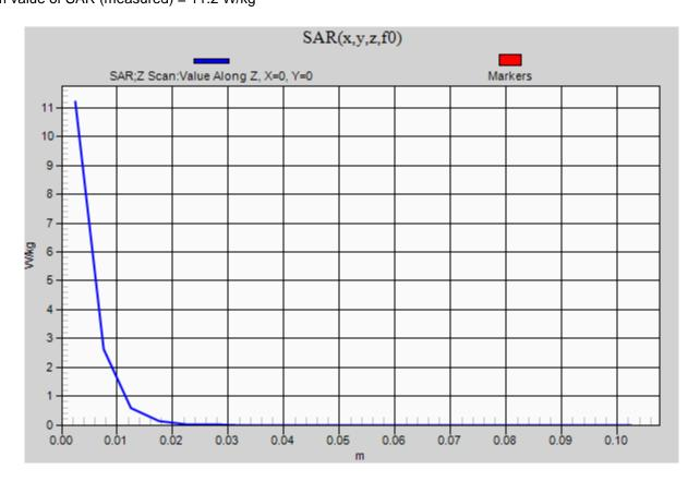
Frequency: 5600 MHz; Duty Cycle: 1:1; Room Ambient Temperature: 24.0°C; Liquid Temperature: 23.0°C Medium parameters used: f = 5600 MHz;  $\sigma$  = 5.045 S/m;  $\epsilon_r$  = 35.089;  $\rho$  = 1000 kg/m<sup>3</sup> DASY5 Configuration:
