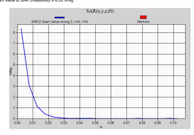
Frequency: 2300 MHz; Duty Cycle: 1:1; Room Ambient Temperature: 24.0°C; Liquid Temperature: 23.0°C Medium parameters used: f = 2300 MHz;  $\sigma$  = 1.666 S/m;  $\epsilon_r$  = 38.878;  $\rho$  = 1000 kg/m<sup>3</sup> DASY5 Configuration:
