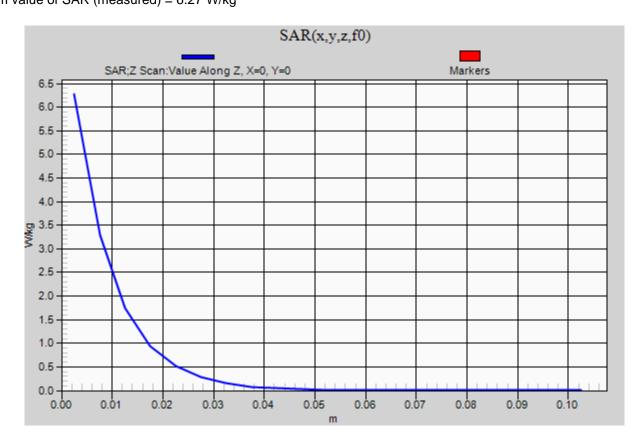
Frequency: 2600 MHz; Duty Cycle: 1:1; Room Ambient Temperature: 24.0°C; Liquid Temperature: 23.0°C Medium parameters used: f = 2600 MHz;  $\sigma$  = 2.008 S/m;  $\epsilon_r$  = 37.813;  $\rho$  = 1000 kg/m<sup>3</sup> DASY5 Configuration:
