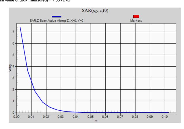
Frequency: 3500 MHz; Duty Cycle: 1:1; Room Ambient Temperature: 24.0°C; Liquid Temperature: 23.0°C Medium parameters used: f = 3500 MHz;  $\sigma$  = 2.798 S/m;  $\epsilon_r$  = 39.736;  $\rho$  = 1000 kg/m<sup>3</sup> DASY5 Configuration:
