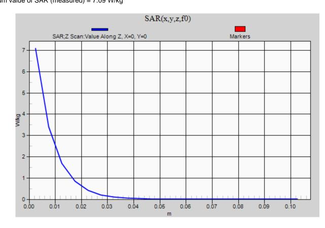
Frequency: 2300 MHz; Duty Cycle: 1:1; Room Ambient Temperature: 24.0°C; Liquid Temperature: 23.0°C Medium parameters used: f = 2300 MHz;  $\sigma$  = 1.727 S/m;  $\epsilon_r$  = 40.485;  $\rho$  = 1000 kg/m<sup>3</sup> DASY5 Configuration:
