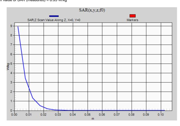
Frequency: 3700 MHz; Duty Cycle: 1:1; Room Ambient Temperature: 24.0°C; Liquid Temperature: 23.0°C Medium parameters used: f = 3700 MHz;  $\sigma$  = 2.986 S/m;  $\epsilon_r$  = 39.406;  $\rho$  = 1000 kg/m<sup>3</sup> DASY5 Configuration:
