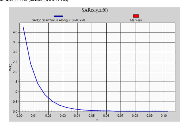
Frequency: 2450 MHz; Duty Cycle: 1:1; Room Ambient Temperature: 24.0°C; Liquid Temperature: 23.0°C Medium parameters used: f = 2450 MHz;  $\sigma$  = 1.731 S/m;  $\epsilon_r$  = 38.253;  $\rho$  = 1000 kg/m<sup>3</sup> DASY5 Configuration:
