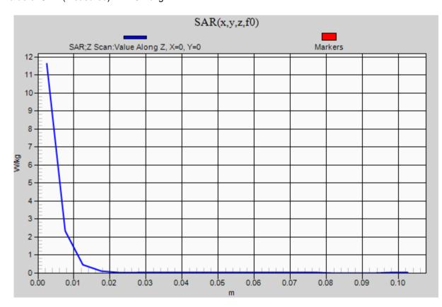
Frequency: 5250 MHz; Duty Cycle: 1:1; Room Ambient Temperature: 24.0°C; Liquid Temperature: 23.0°C Medium parameters used: f = 5250 MHz;  $\sigma$  = 4.586 S/m;  $\epsilon_r$  = 34.735;  $\rho$  = 1000 kg/m<sup>3</sup> DASY5 Configuration:
