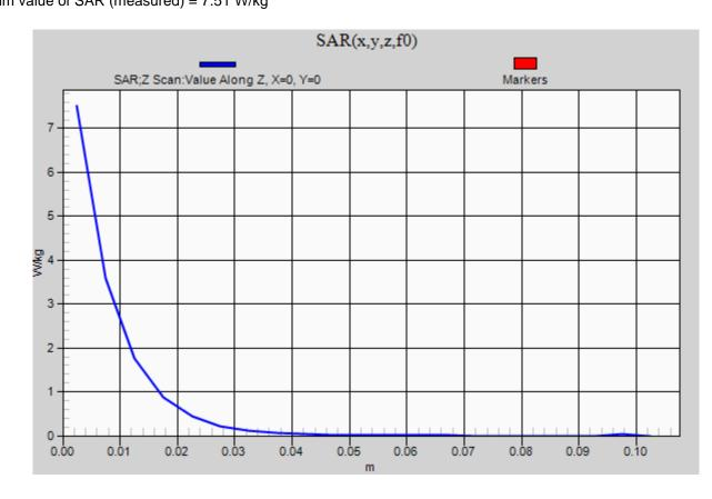
Frequency: 3500 MHz; Duty Cycle: 1:1; Room Ambient Temperature: 24.0°C; Liquid Temperature: 23.0°C Medium parameters used: f = 3500 MHz;  $\sigma$  = 2.849 S/m;  $\epsilon_r$  = 39.267;  $\rho$  = 1000 kg/m<sup>3</sup> DASY5 Configuration:
