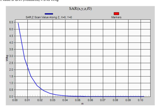
Frequency: 3500 MHz; Duty Cycle: 1:1; Room Ambient Temperature: 24.0°C; Liquid Temperature: 23.0°C Medium parameters used: f = 3500 MHz;  $\sigma$  = 2.778 S/m;  $\epsilon_r$  = 38.921;  $\rho$  = 1000 kg/m<sup>3</sup> DASY5 Configuration:
