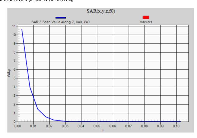
Frequency: 1900 MHz; Duty Cycle: 1:1; Room Ambient Temperature: 24.0°C; Liquid Temperature: 23.0°C Medium parameters used: f = 1900 MHz;  $\sigma$  = 1.432 S/m;  $\epsilon_r$  = 38.972;  $\rho$  = 1000 kg/m<sup>3</sup> DASY5 Configuration:
