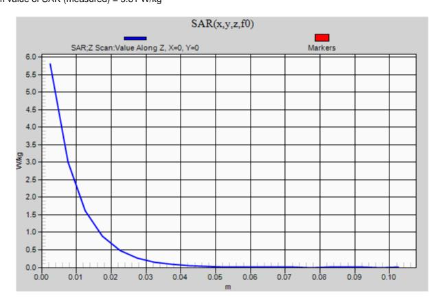
Frequency: 2450 MHz; Duty Cycle: 1:1; Room Ambient Temperature: 24.0°C; Liquid Temperature: 23.0°C Medium parameters used: f = 2450 MHz;  $\sigma$  = 1.774 S/m;  $\epsilon_r$  = 39.667;  $\rho$  = 1000 kg/m<sup>3</sup> DASY5 Configuration:
