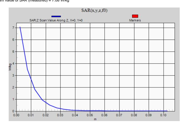
Frequency: 750 MHz; Duty Cycle: 1:1; Room Ambient Temperature: 24.0°C; Liquid Temperature: 23.0°C Medium parameters used: f = 750 MHz;  $\sigma$  = 0.891 S/m;  $\epsilon_r$  = 40.202;  $\rho$  = 1000 kg/m<sup>3</sup> DASY5 Configuration:
