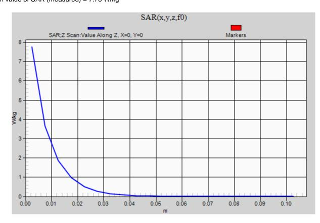
Frequency: 2450 MHz; Duty Cycle: 1:1; Room Ambient Temperature: 24.0°C; Liquid Temperature: 23.0°C Medium parameters used: f = 2450 MHz;  $\sigma$  = 1.751 S/m;  $\epsilon_r$  = 38.085;  $\rho$  = 1000 kg/m<sup>3</sup> DASY5 Configuration:
