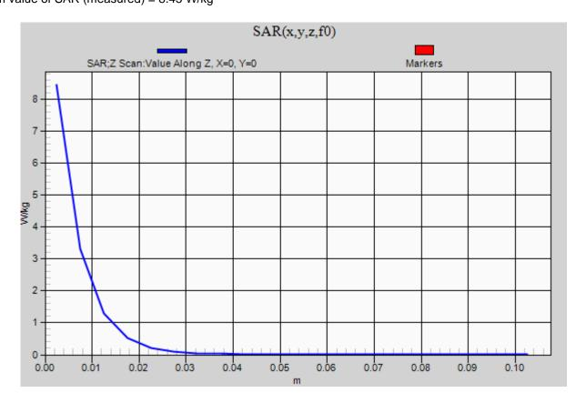
Frequency: 5200 MHz; Duty Cycle: 1:1; Room Ambient Temperature: 24.0°C; Liquid Temperature: 23.0°C Medium parameters used: f = 5200 MHz;  $\sigma$  = 4.464 S/m;  $\epsilon_r$  = 34.973;  $\rho$  = 1000 kg/m<sup>3</sup> DASY5 Configuration:
