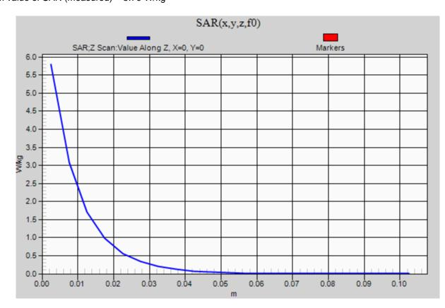
Frequency: 2300 MHz; Duty Cycle: 1:1; Room Ambient Temperature: 24.0°C; Liquid Temperature: 23.0°C Medium parameters used: f = 2300 MHz;  $\sigma$  = 1.712 S/m;  $\epsilon_r$  = 39.447;  $\rho$  = 1000 kg/m<sup>3</sup> DASY5 Configuration:
