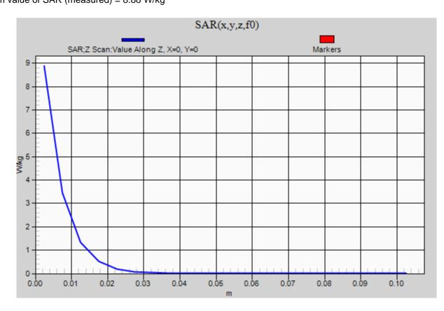
Frequency: 1750 MHz; Duty Cycle: 1:1; Room Ambient Temperature: 24.0°C; Liquid Temperature: 23.0°C Medium parameters used: f = 1750 MHz;  $\sigma$  = 1.41 S/m;  $\epsilon_r$  = 38.99;  $\rho$  = 1000 kg/m<sup>3</sup> DASY5 Configuration:
