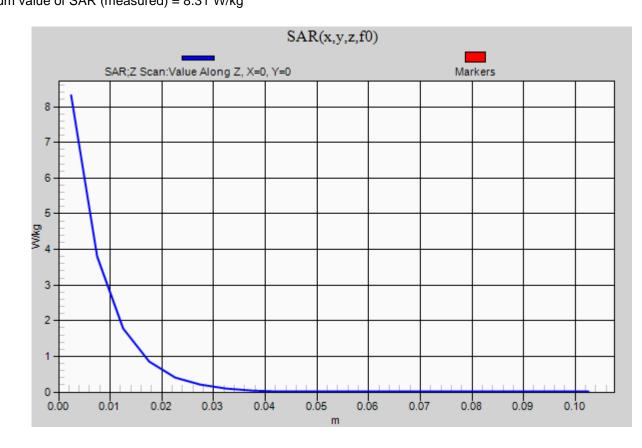
Frequency: 5800 MHz; Duty Cycle: 1:1; Room Ambient Temperature: 24.0°C; Liquid Temperature: 23.0°C Medium parameters used: f = 5800 MHz;  $\sigma$  = 5.097 S/m;  $\epsilon_r$  = 36.019;  $\rho$  = 1000 kg/m<sup>3</sup> DASY5 Configuration:
