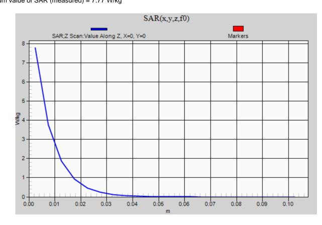
Frequency: 2600 MHz; Duty Cycle: 1:1; Room Ambient Temperature: 24.0°C; Liquid Temperature: 23.0°C Medium parameters used: f = 2600 MHz;  $\sigma$  = 2.026 S/m;  $\epsilon_r$  = 39.988;  $\rho$  = 1000 kg/m<sup>3</sup> DASY5 Configuration:
