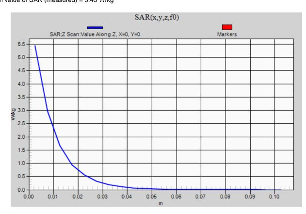
Frequency: 3500 MHz; Duty Cycle: 1:1; Room Ambient Temperature: 24.0°C; Liquid Temperature: 23.0°C Medium parameters used: f = 3500 MHz;  $\sigma$  = 2.82 S/m;  $\epsilon_r$  = 39.704;  $\rho$  = 1000 kg/m<sup>3</sup> DASY5 Configuration:
