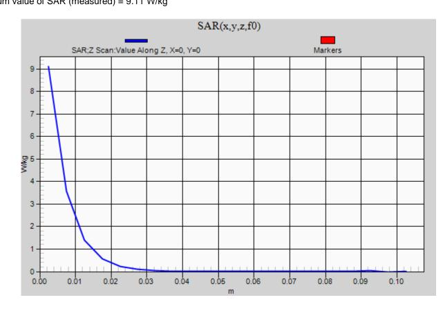
Frequency: 3500 MHz; Duty Cycle: 1:1; Room Ambient Temperature: 24.0°C; Liquid Temperature: 23.0°C Medium parameters used: f = 3500 MHz;  $\sigma$  = 2.896 S/m;  $\epsilon_r$  = 39.398;  $\rho$  = 1000 kg/m<sup>3</sup> DASY5 Configuration:
