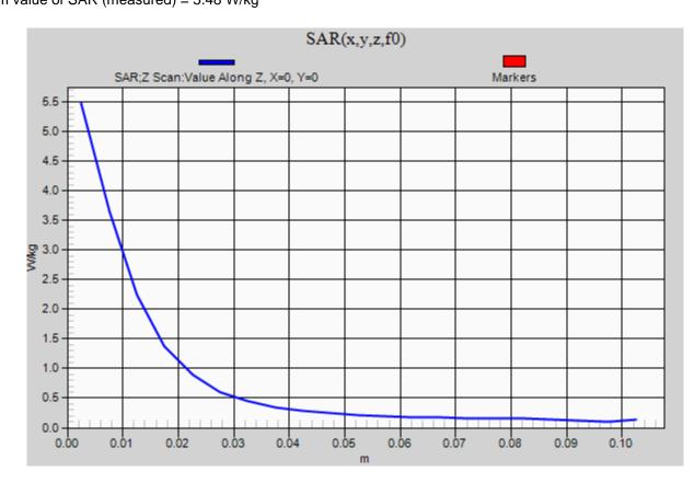
Frequency: 2600 MHz; Duty Cycle: 1:1; Room Ambient Temperature: 24.0°C; Liquid Temperature: 23.0°C Medium parameters used: f = 2600 MHz;  $\sigma$  = 1.922 S/m;  $\epsilon_r$  = 39.348;  $\rho$  = 1000 kg/m<sup>3</sup> DASY5 Configuration:
