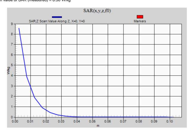
Frequency: 1750 MHz; Duty Cycle: 1:1; Room Ambient Temperature: 24.0°C; Liquid Temperature: 23.0°C Medium parameters used: f = 1750 MHz;  $\sigma$  = 1.339 S/m;  $\epsilon_r$  = 38.804;  $\rho$  = 1000 kg/m<sup>3</sup> DASY5 Configuration:
