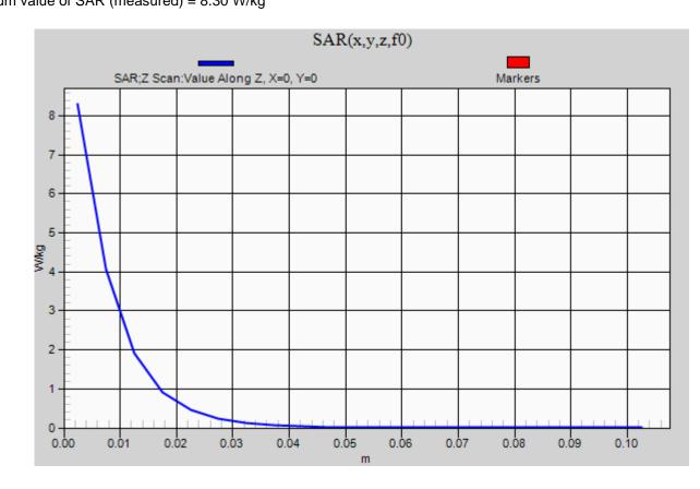
Frequency: 2450 MHz; Duty Cycle: 1:1; Room Ambient Temperature: 24.0°C; Liquid Temperature: 23.0°C Medium parameters used: f = 2450 MHz;  $\sigma$  = 1.879 S/m;  $\epsilon_r$  = 38.111;  $\rho$  = 1000 kg/m<sup>3</sup> DASY5 Configuration:
