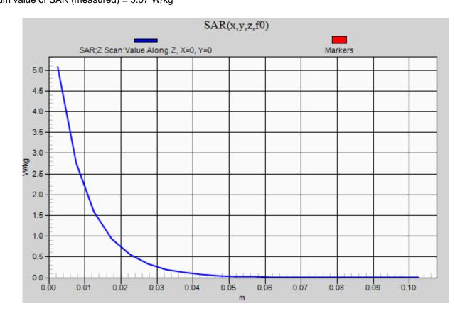
Frequency: 5600 MHz; Duty Cycle: 1:1; Room Ambient Temperature: 24.0°C; Liquid Temperature: 23.0°C Medium parameters used: f = 5600 MHz;  $\sigma$  = 4.953 S/m;  $\epsilon_r$  = 34.478;  $\rho$  = 1000 kg/m<sup>3</sup> DASY5 Configuration:
