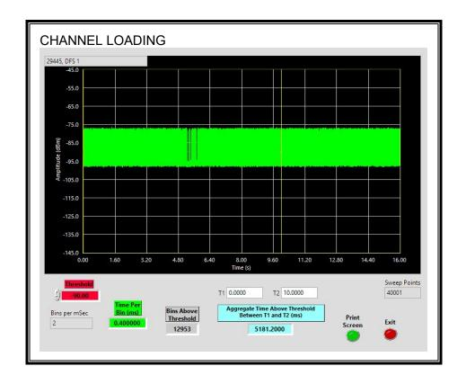
The level of traffic loading on the channel by the EUT is 51.81%
