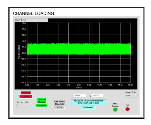
The level of traffic loading on the channel by the EUT is 30.93%
