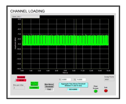
The level of traffic loading on the channel by the EUT is 30.24%
