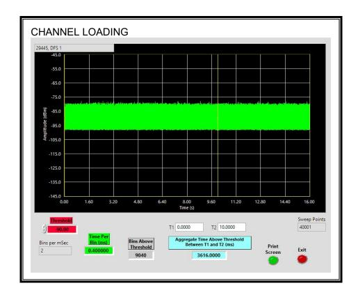
The level of traffic loading on the channel by the EUT is 36.16%
