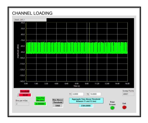
The level of traffic loading on the channel by the EUT is 23.84%
