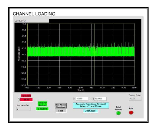
The level of traffic loading on the channel by the Peer Slave is 20.04%
