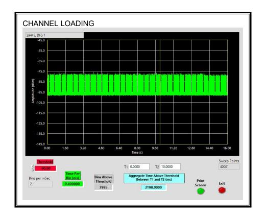
The level of traffic loading on the channel by the EUT is 31.98%
