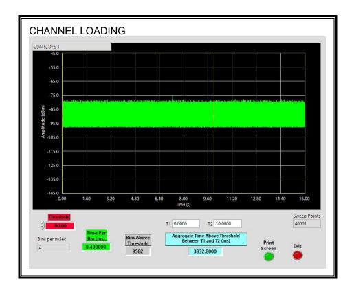
The level of traffic loading on the channel by the EUT is 38.32%
