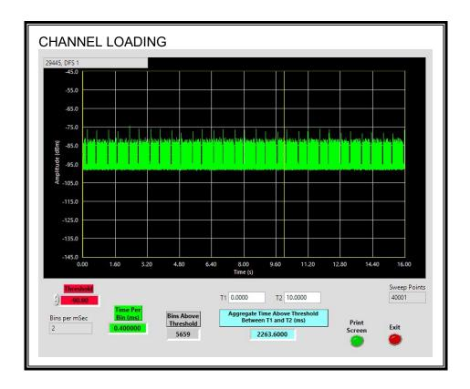
The level of traffic loading on the channel by the Peer Slave is 22.63%
