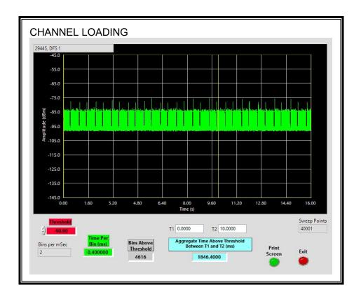
The level of traffic loading on the channel by the Peer Slave is 18.46%
