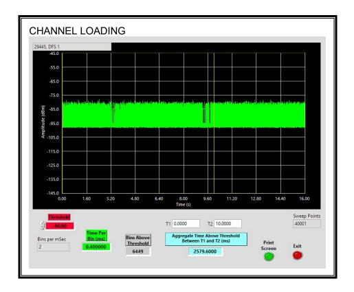
The level of traffic loading on the channel by the EUT is 25.79%
