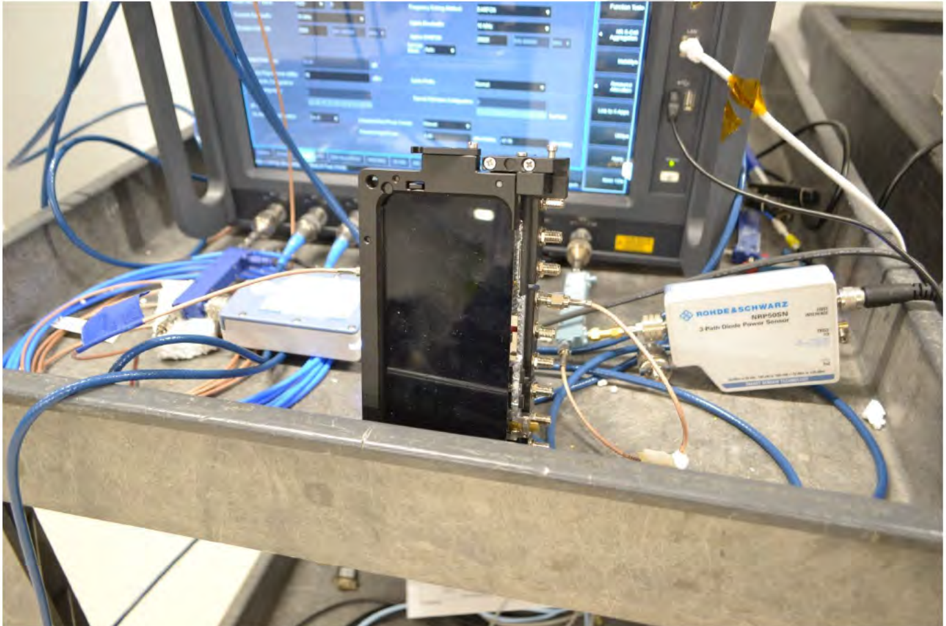
Figure C-3 UXM Conducted power test measurement setup dual port
