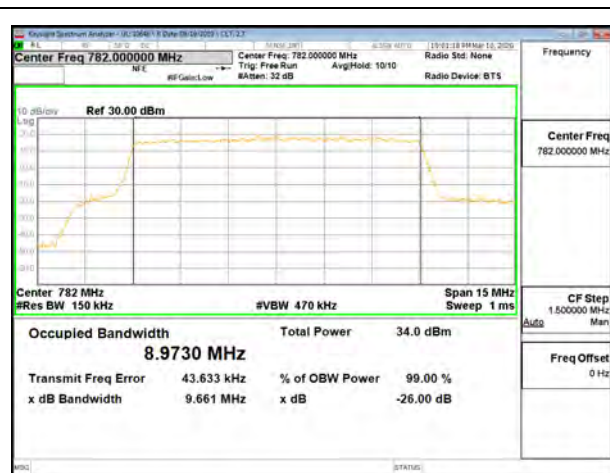
LTE B13 10MHz QPSK Middle Channel RB50-0
