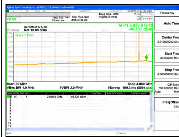
LTE B48 15MHz QPSK Mid Channel RB1-0 (30MHz to 4GHz)
