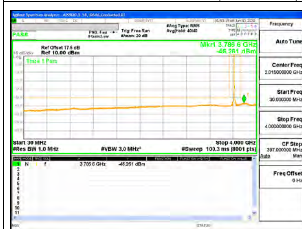
LTE B48 5MHz QPSK Mid Channel RB1-0 (30MHz to 4GHz)
