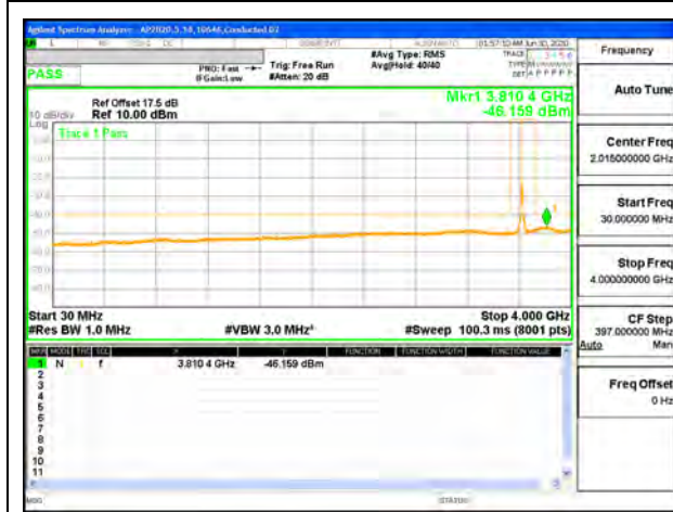
LTE B48 10MHz QPSK Mid Channel RB1-0 (30MHz to 4GHz)
