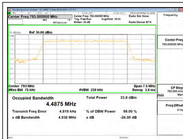
LTE B14 5MHz QPSK Middle Channel RB25-0
