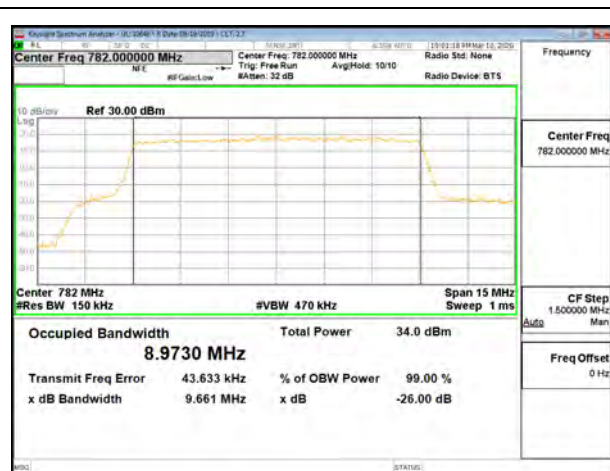
LTE B13 10MHz QPSK Middle Channel RB50-0
