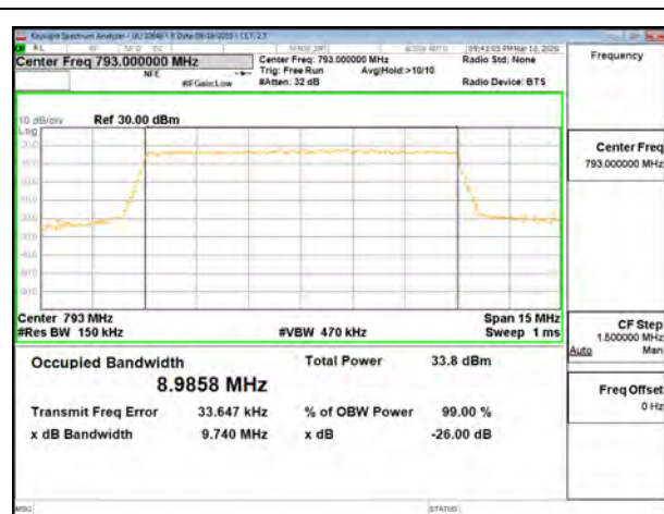
LTE B14 10MHz QPSK Middle Channel RB50-0
